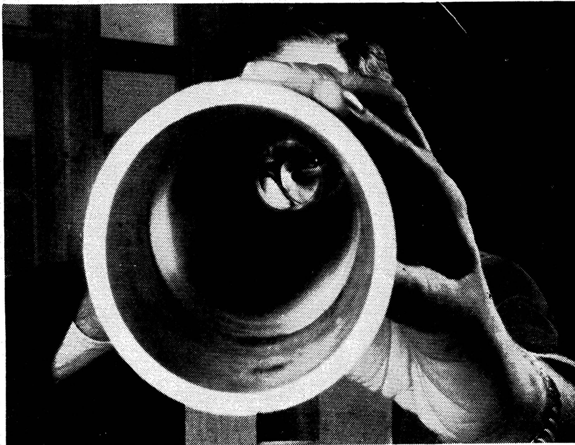
A LOOK INTO THE FUTURE —The hollow tube, held by a Bell Telephone Laboratories engineer, is an experimental Waveguide for telephone service and television. It's not as large as it looks here. (Actually, only two inches in diameter.) Some day it may be no thicker than a fountain pen.
