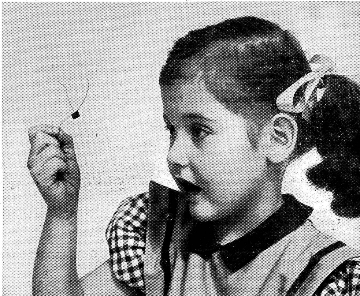
THAT'S A TRANSISTOR, invented at Bell Telephone Laboratories. This tiny electronic device can do many things that vacuum tubes can do and more besides. Though little larger than a coffee bean, it can amplify electric signals 100,000 times.
