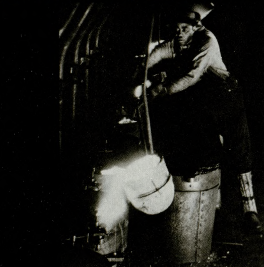
Man pouring hot metal into molds, Ford Motor Company, River Rouge Plant, Dearborn, Michigan, 1933. (Photo courtesy Henry Ford Museum and Greenfield Village, Dearborn, Michigan)
