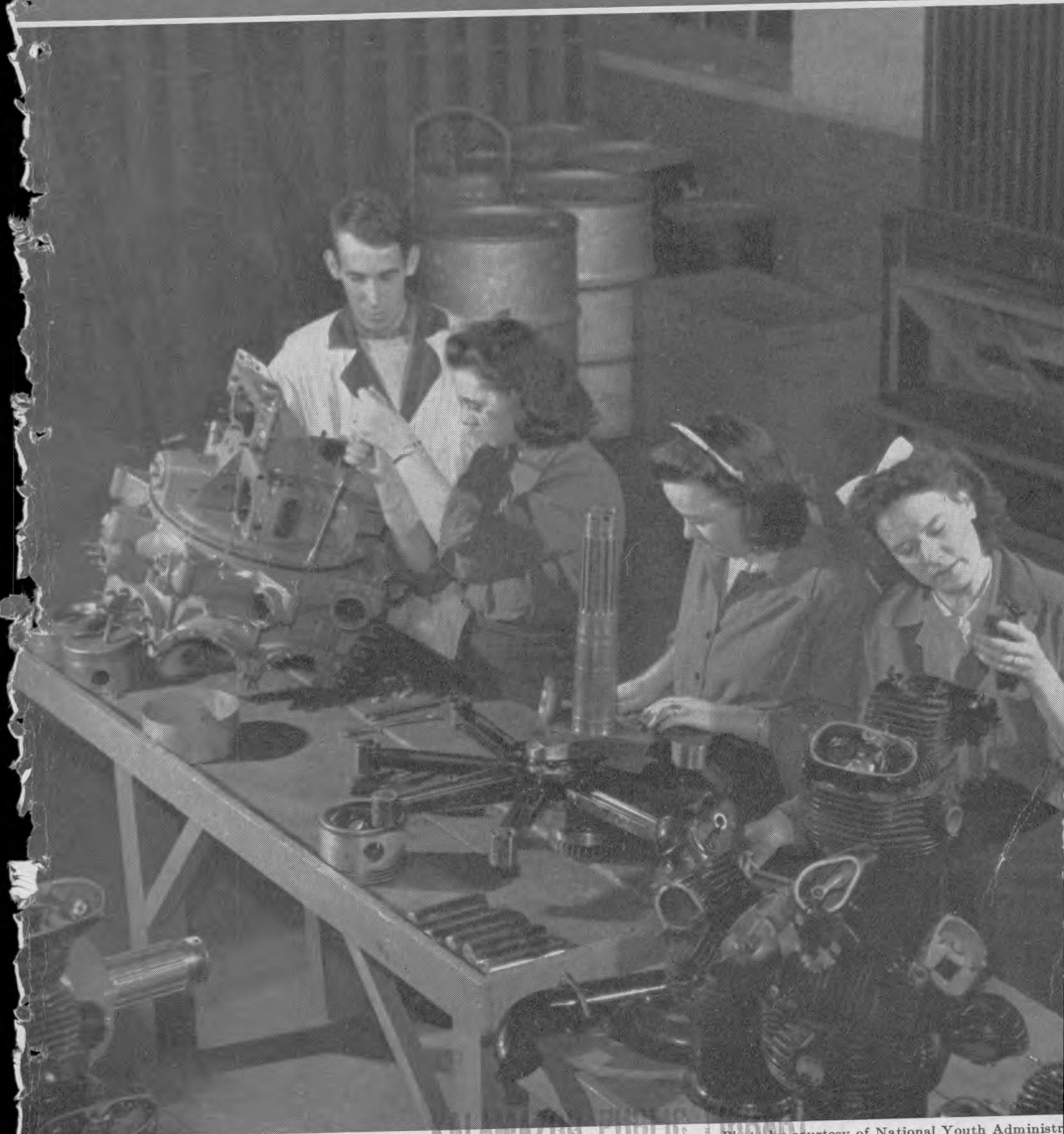
KALAMAZOO PUBLIC LIBRARY Photo by courtesy of National Youth Administration Learning to Repair and Check Airplane Motors
