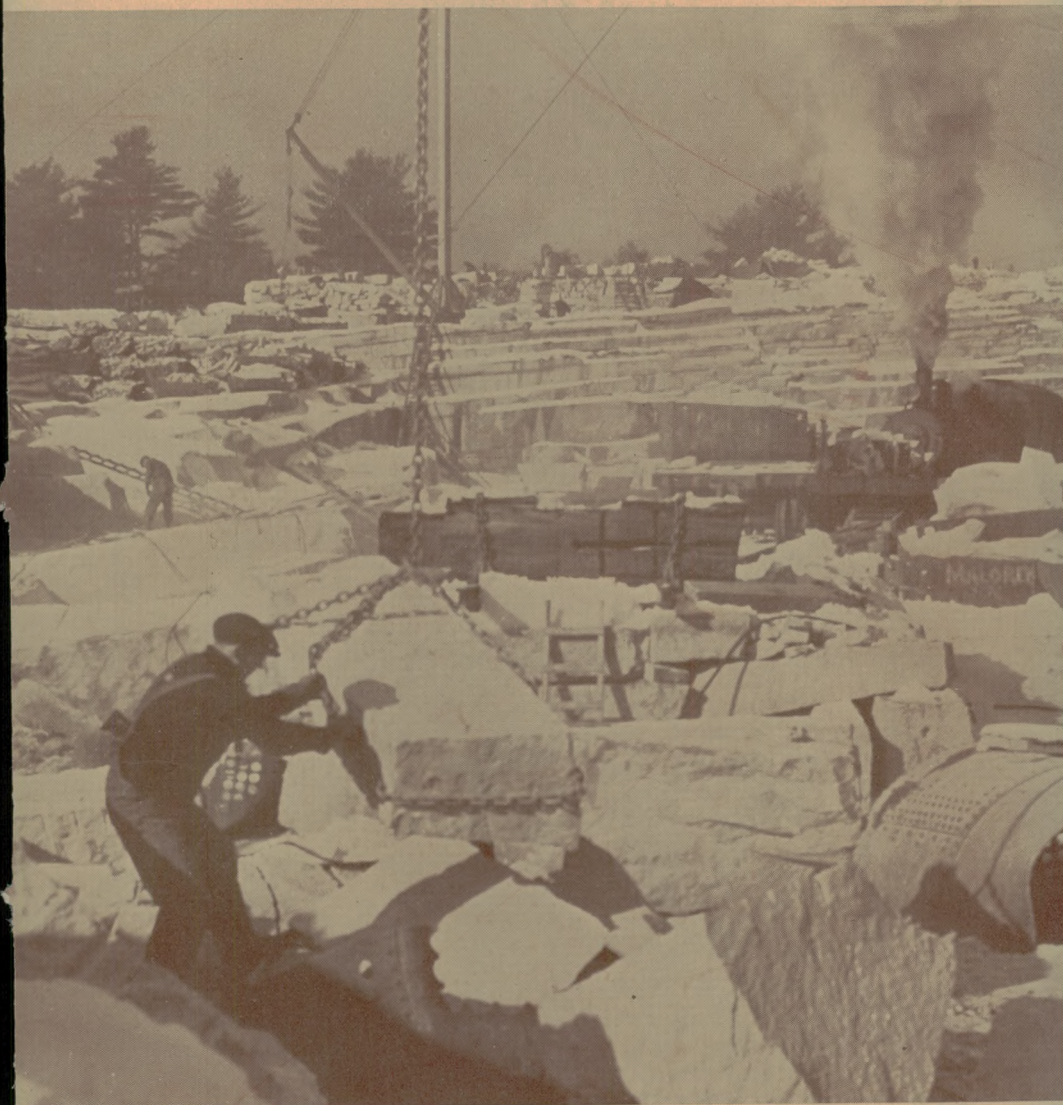
Loading Large Blocks in Granite Quarry
