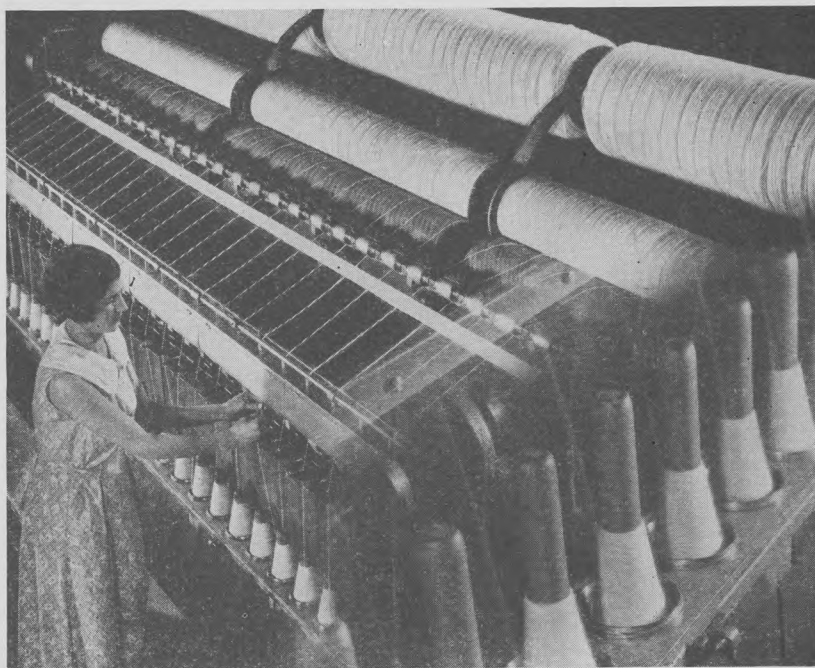
FIGURE 4.—ON RING SPINNING FRAMES THE OPERATION IS CONTINUOUS AND BOBBINS ARE SEVERAL TIMES AS LARGE AS THOSE USED ON MULE.
