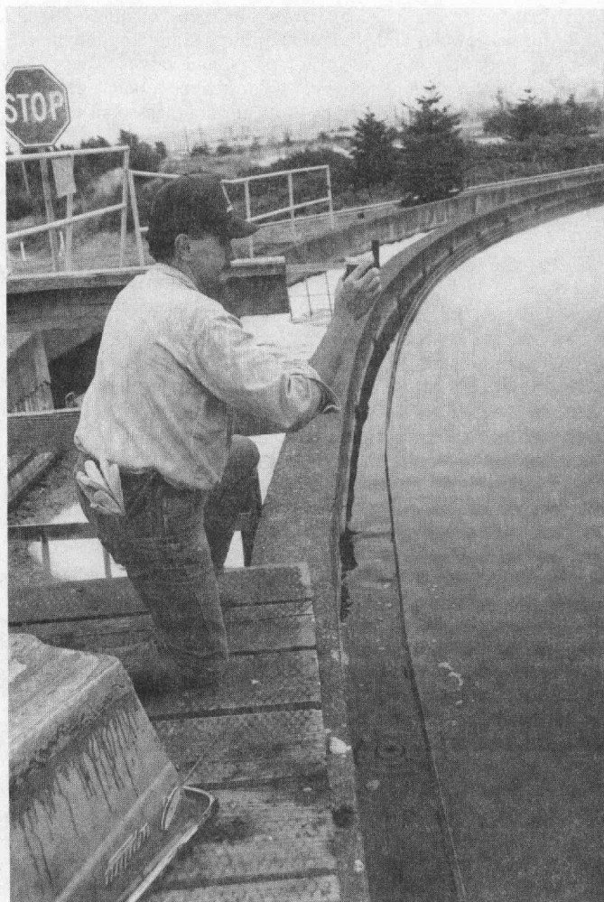
Wastewater treatment plant operators take samples frequently to measure levels of contaminants.
