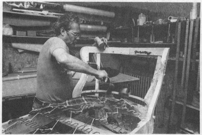
Upholsterers use common handtools, including tack hammers, to make or recondition furniture.
