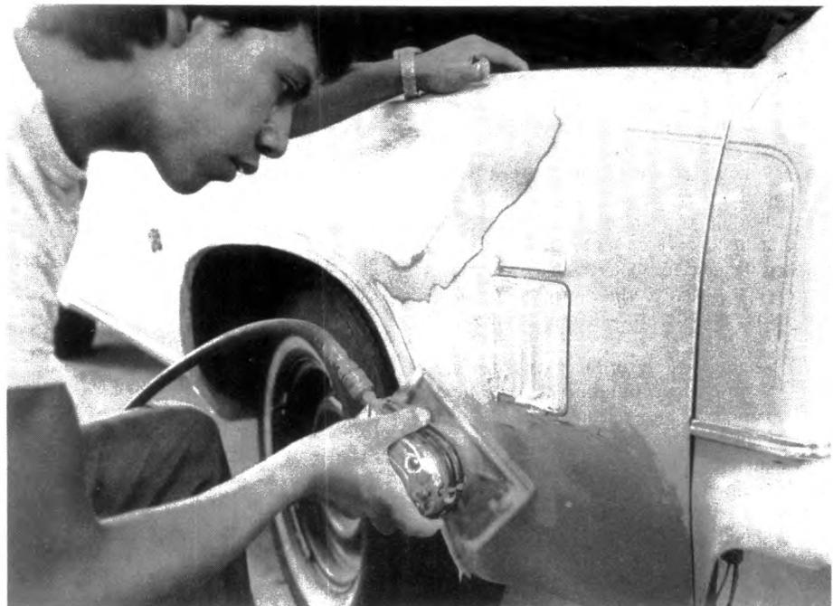
Auto body repairers fill small dents with plastic or solder and then sand the surface.
