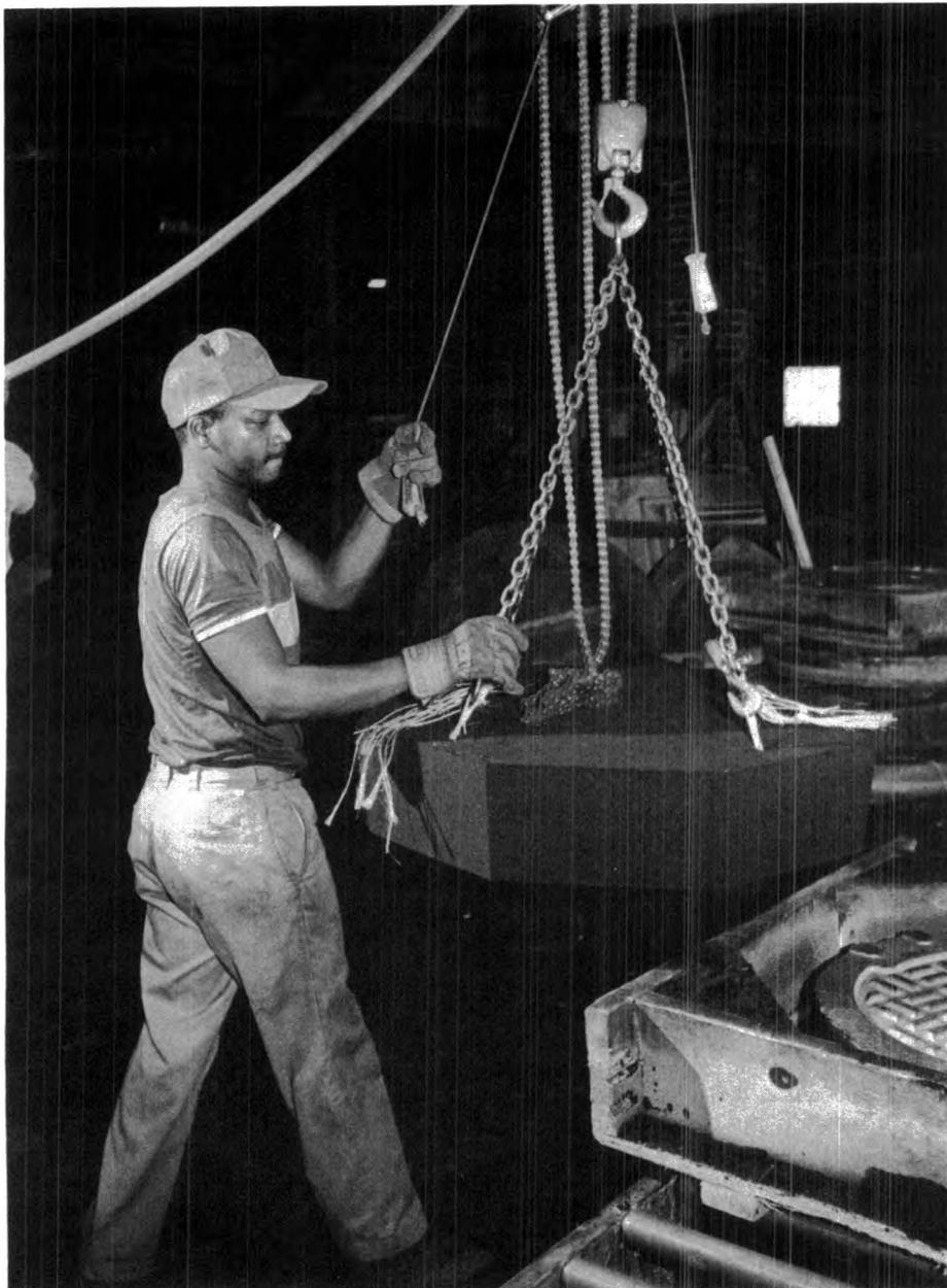
Coremakers prepare the "cores" that form the hollow sections of industrial equipment.
