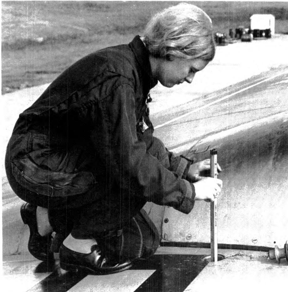
Technician checks an aircraft's fuel supply.
