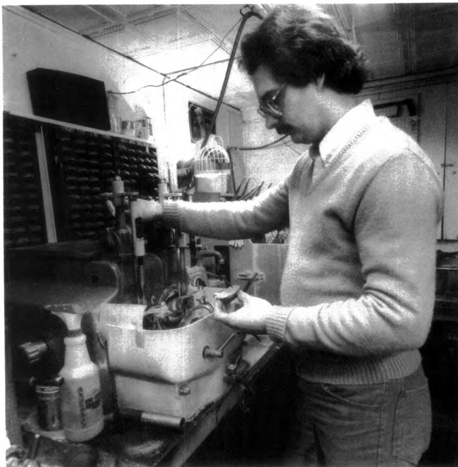
Ophthalmic laboratory technicians operate machines that grind and polish lenses.
