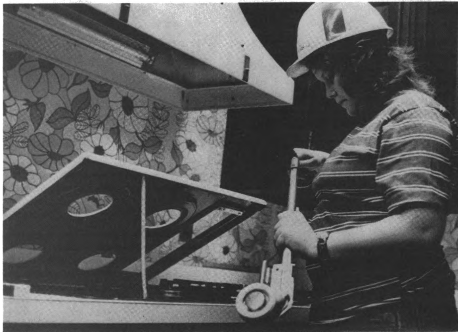
An appliance repairer cleaning the burner of a gas range.
