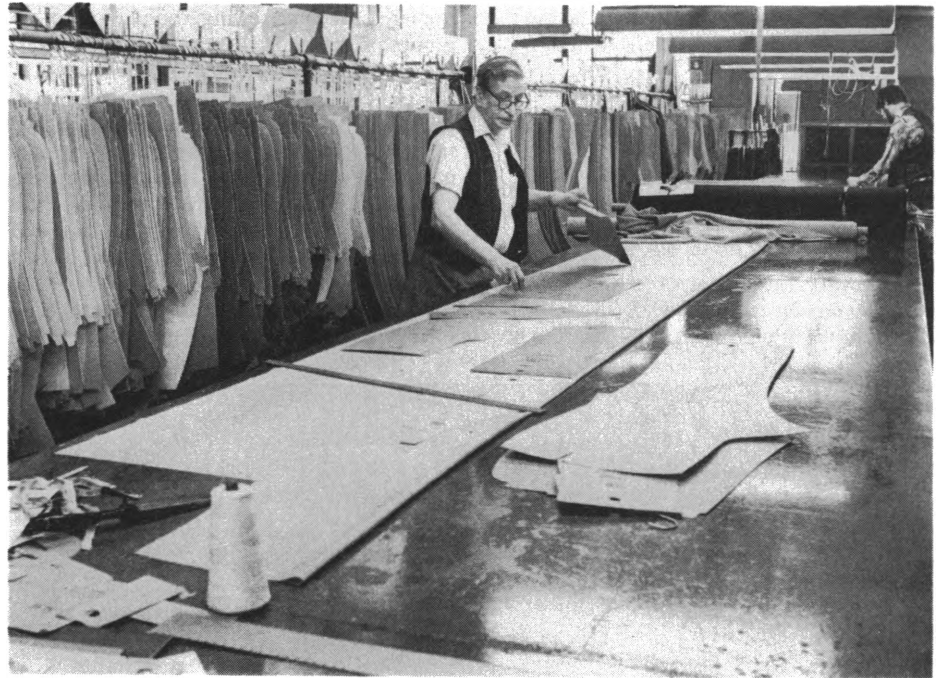
Markers arrange pattern pieces to get the greatest number of garments from the smallest quantity of cloth.
