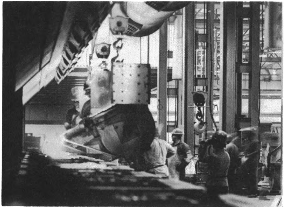
When large numbers of identical castings are needed, high-production molding machines are used.
