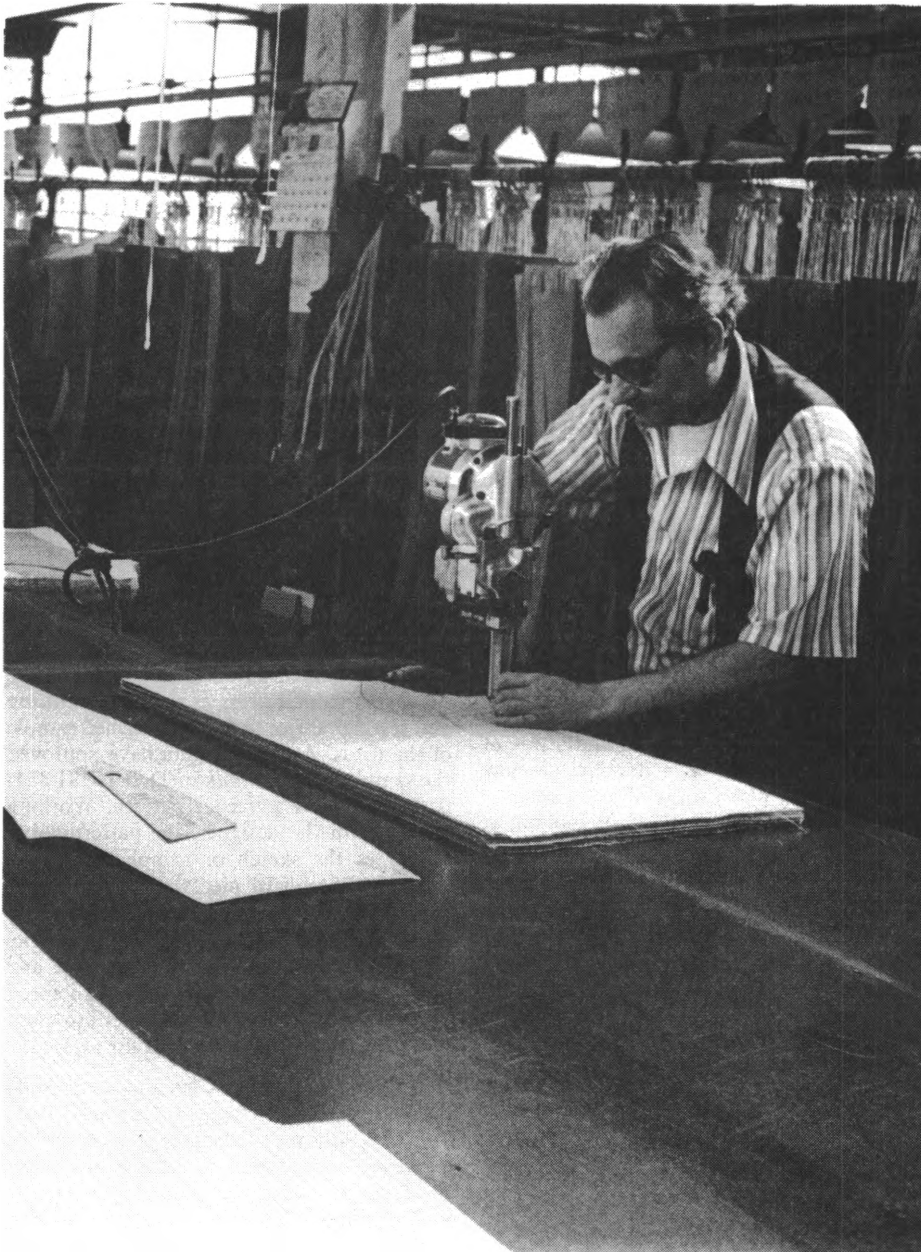
Following the patterns outlined on the cloth, a cutter cuts out garment pieces from layers of cloth.
