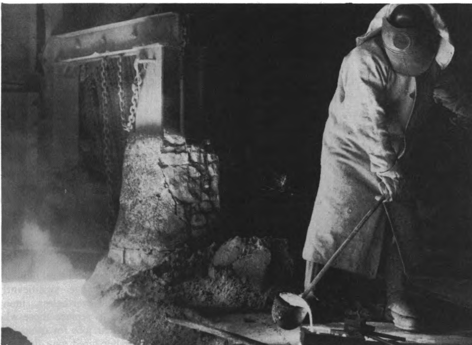
Covered with protective clothing, a worker takes a sample of molten iron.
