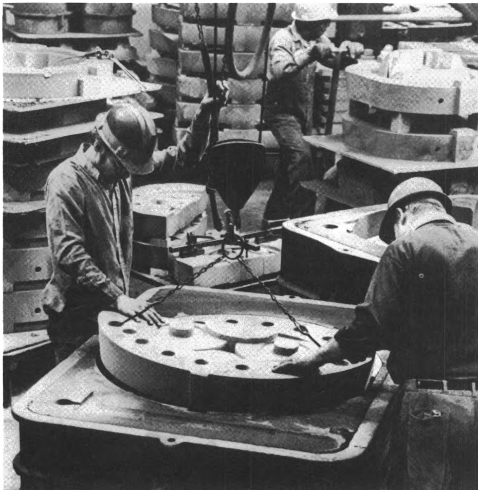
Cores must be carefully positioned into molds to produce an accurate casting.
