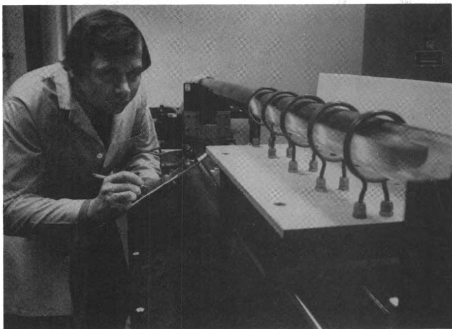
Physicist "growing" germanium crystals in a laboratory.
