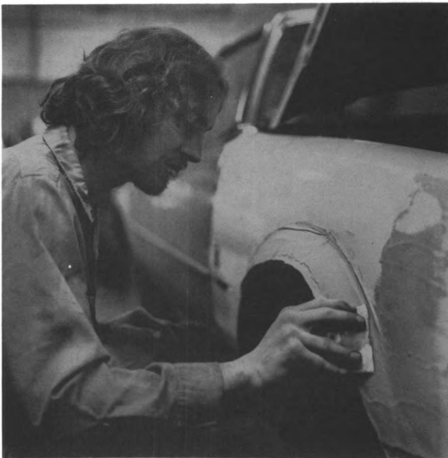
Automobile body repairers fill small dents with plastic and then sand the surface smooth.
