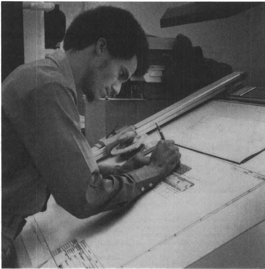
In preparing drawings, drafters use rulers, triangles, and other drafting devices.
