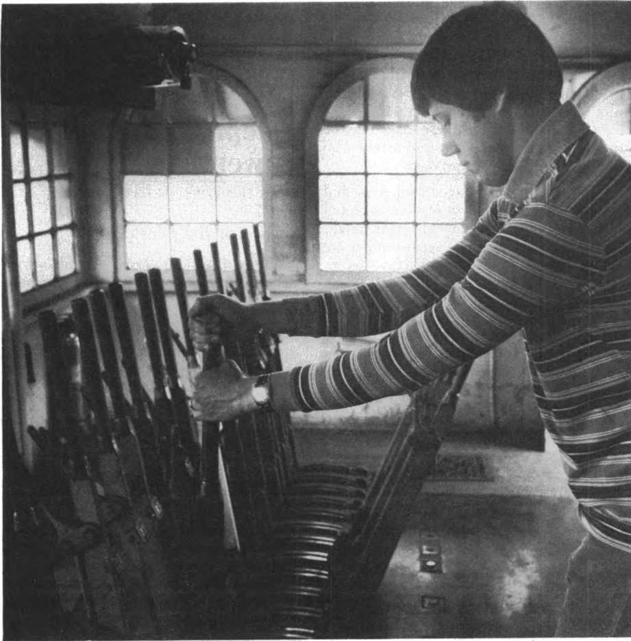
Tower operator uses controls to throw switches on the tracks below.
