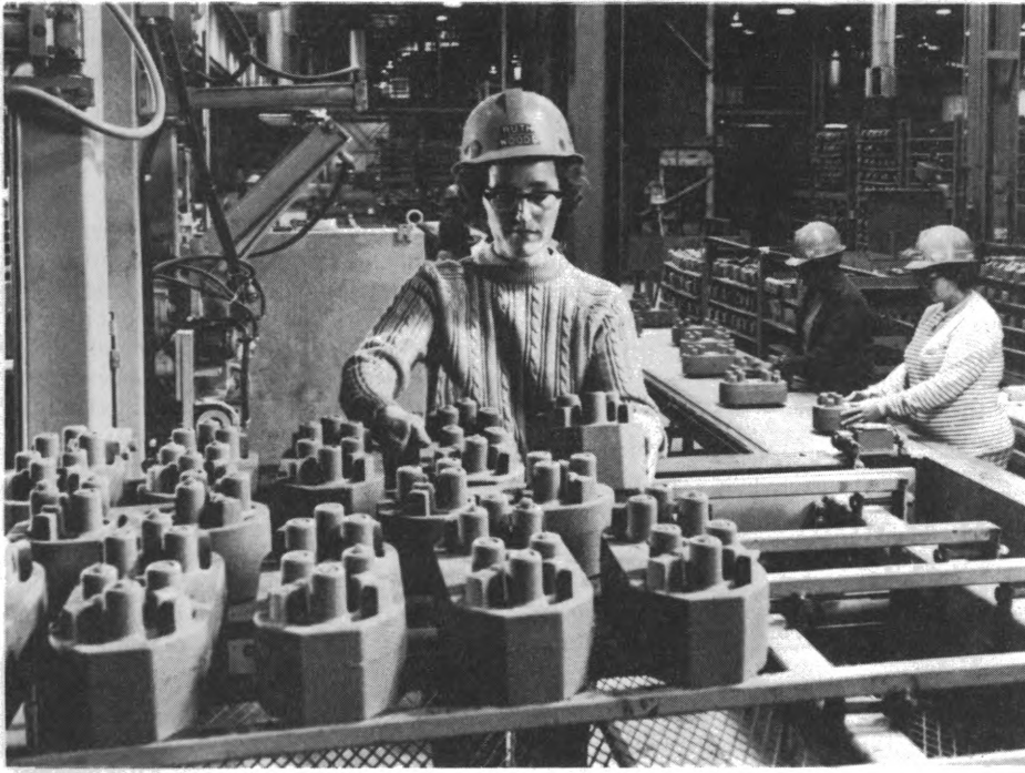
Coremakers prepare the "cores" that form the hollow sections for automobile engine blocks.
