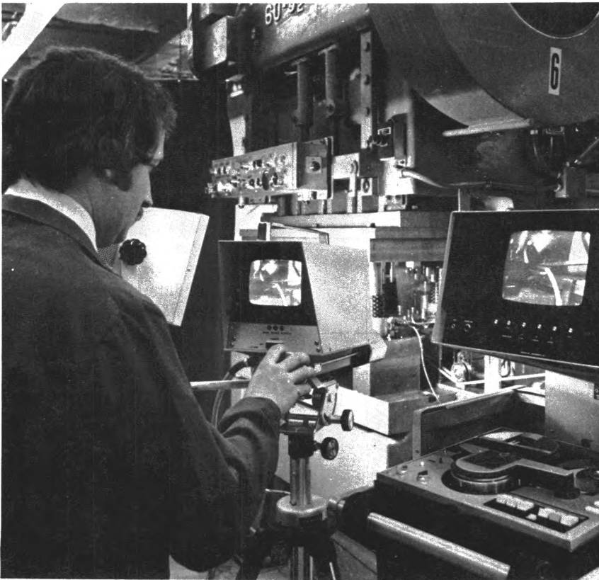
Industrial engineer reviews film of production process to check for problems.
