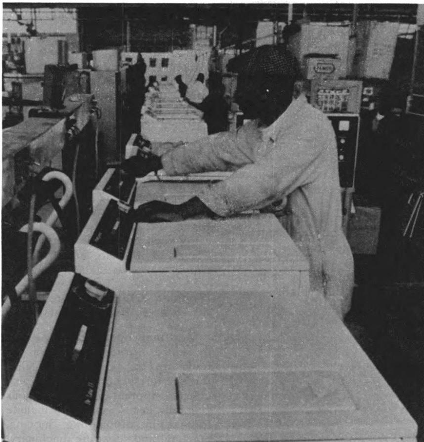
Inspector checks operation of washing machines.
