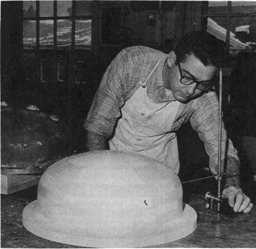
Patternmaker checks dimensions of wooden pattern.
