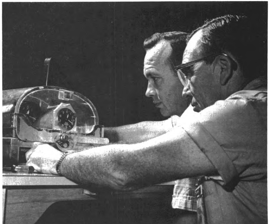
Instrument repairer adjusts vacuum control.
