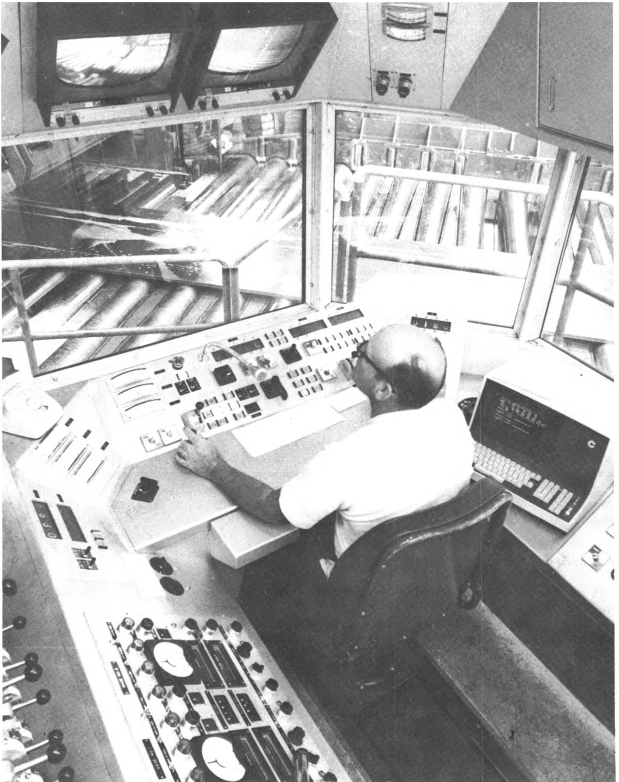
Operator receives a continuous readout of data from the computer during the processing of aluminum plate.
