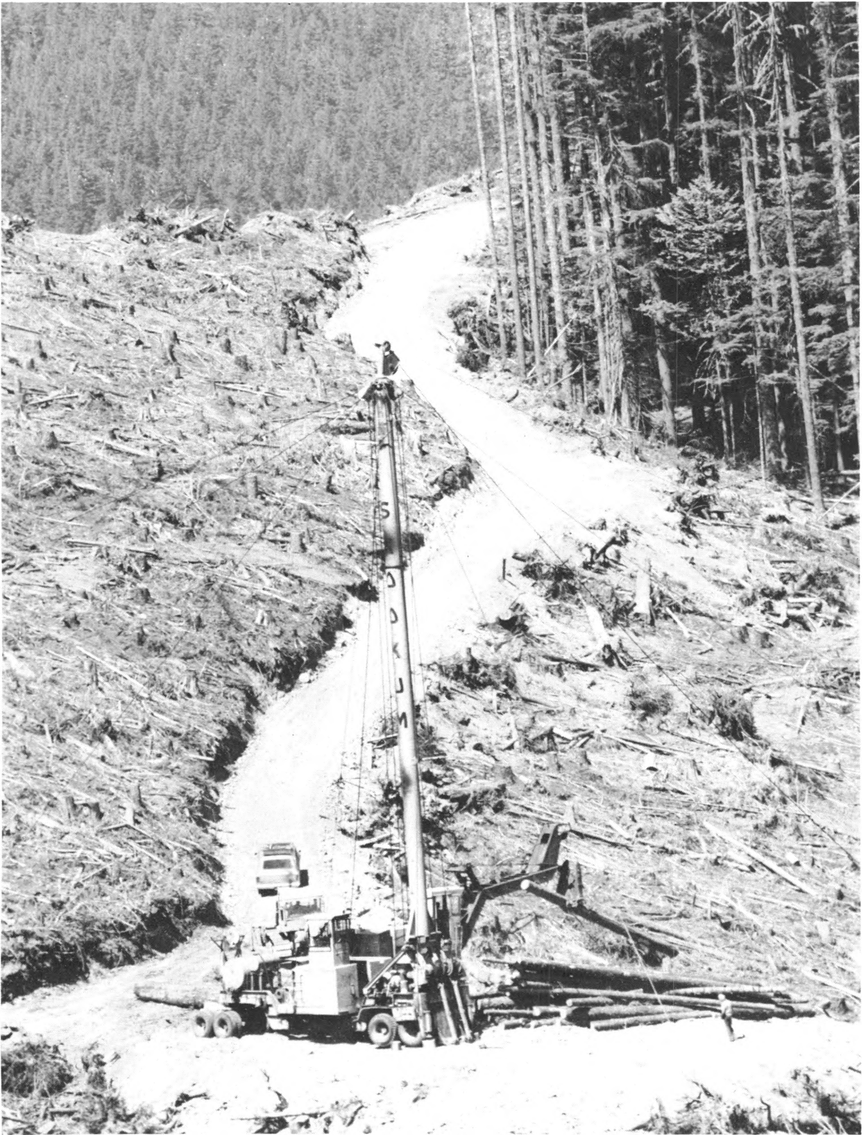
Portable steel spar is used to assemble logs at a central loading point for shipment to the mills.
