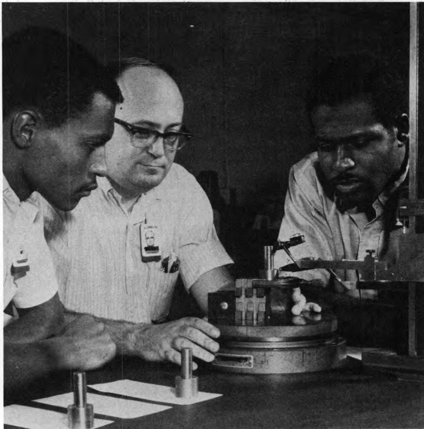
Inspector shows trainees how to check machined parts.
