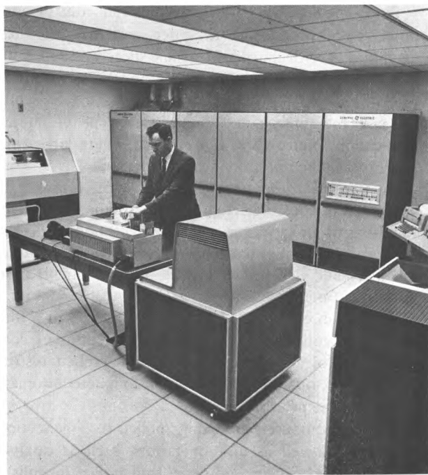
1. Components of a process computer system, including main frame, disc memory, card punch and reader, printer, printout typewriters, and signal terminal cabinets.
