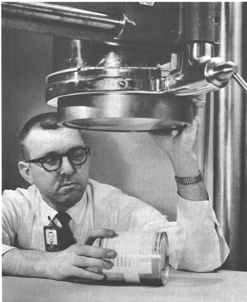
Health physicist positions can of paint under gamma scintillation counter before monitoring its radiation content.
