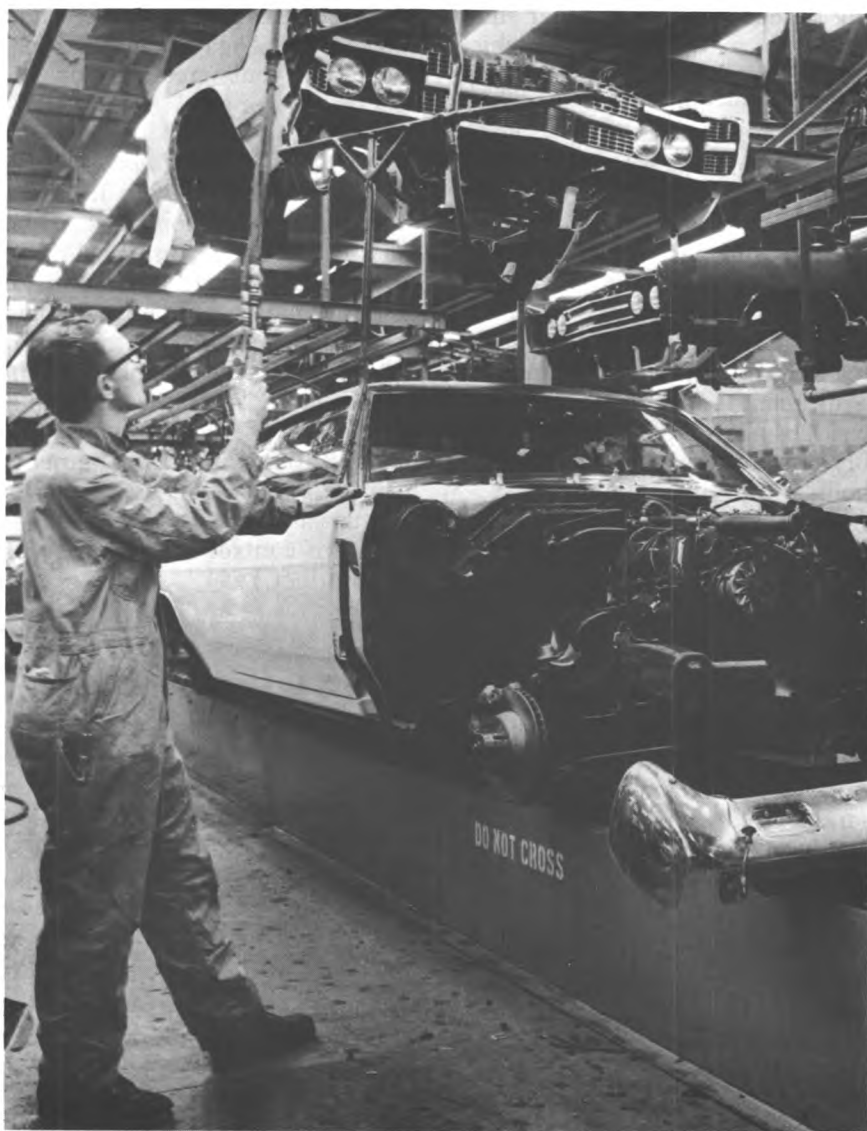
Employees lower front and subassembly into place.
