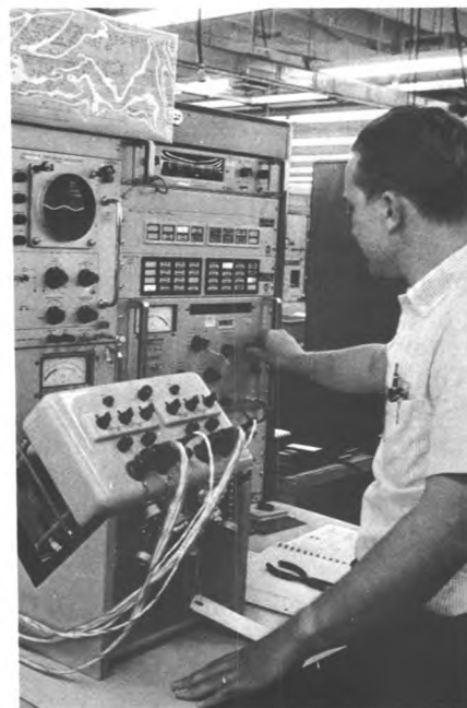
Inspector tests power supply module.
