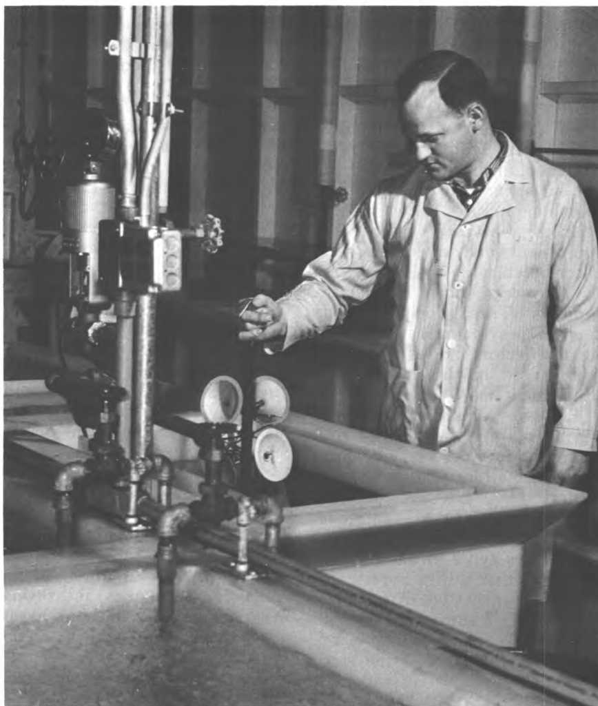
Electroplater inspects batch of plastic items immersed in nickel solution.
