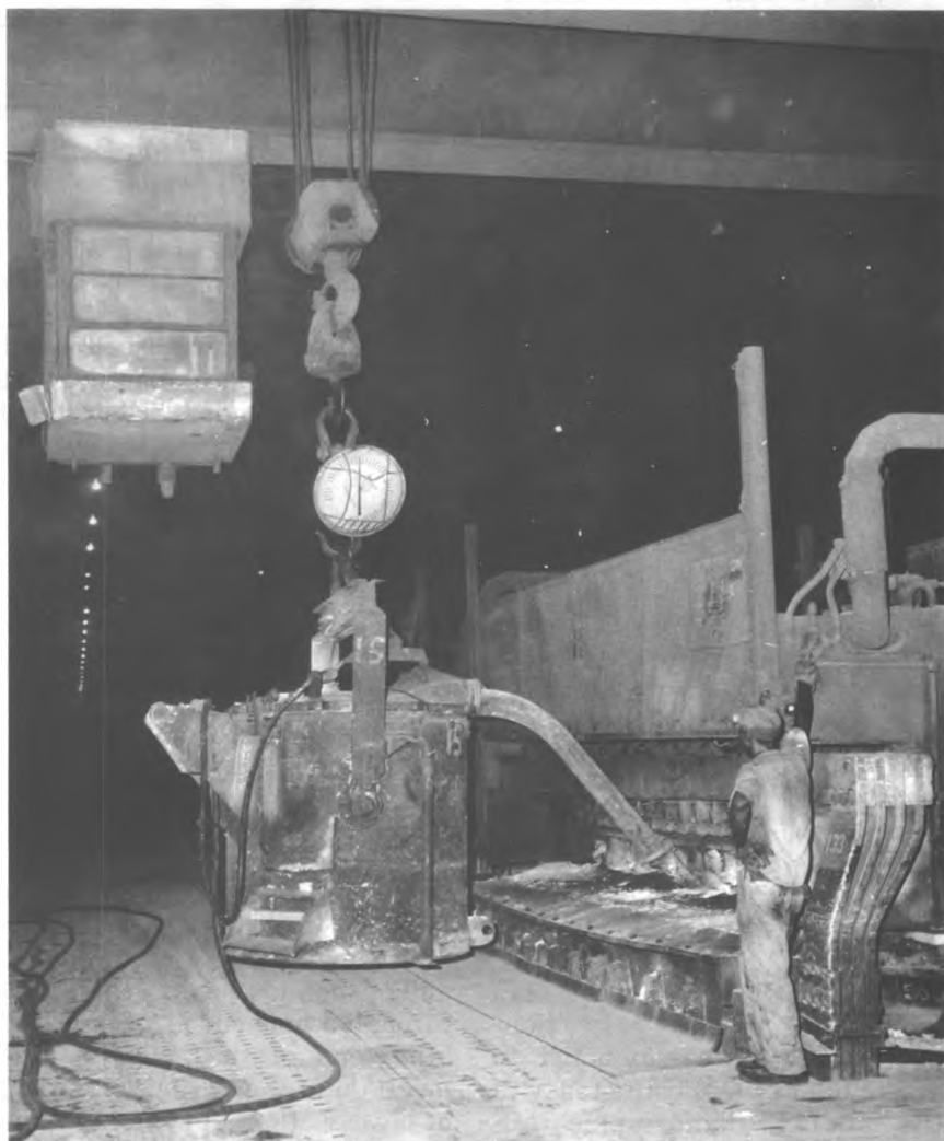
Aluminum is tapped into crucible.
