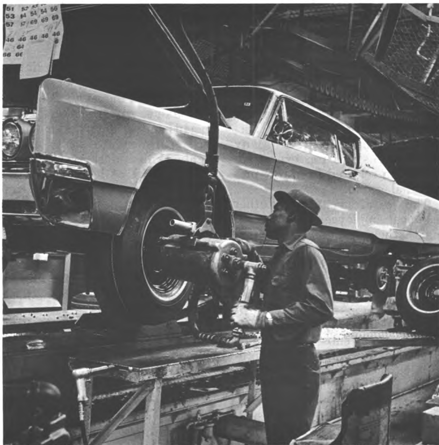
Assembly line employee mounts wheels and tires with impact wrench.
