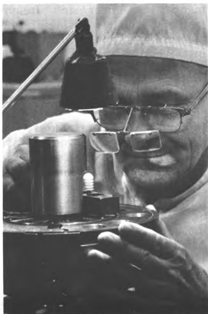
Precision assembler measures and recesses computer recording heads.
