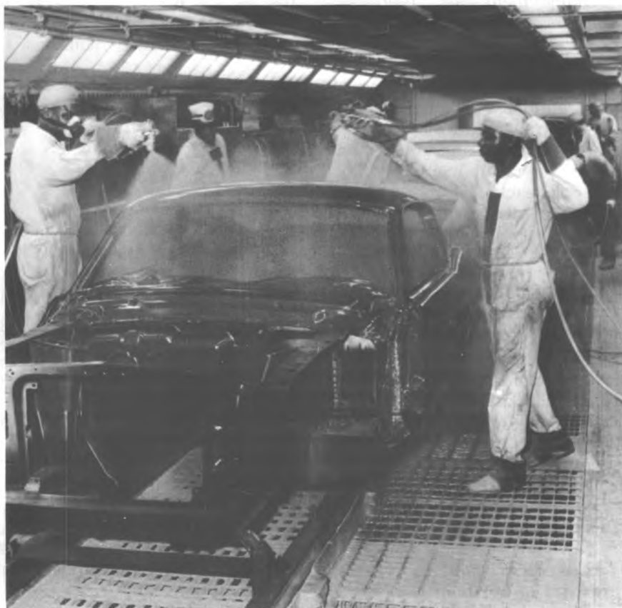
Production painters apply acrylic enamel to automobile body.
