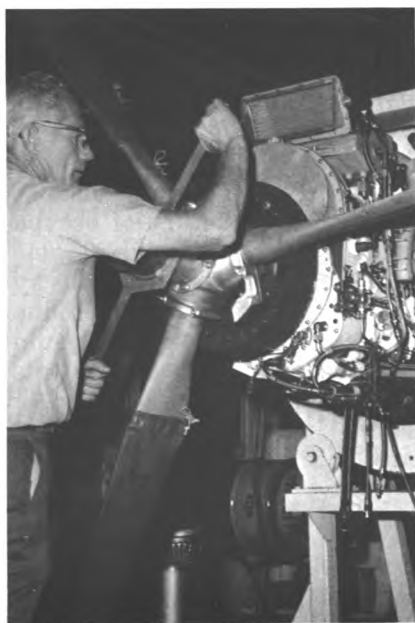
Engine installer makes propeller adjustments.
