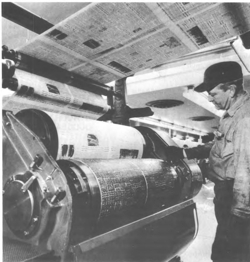
Pressman adjusts stereotype plate on newspaper press.
