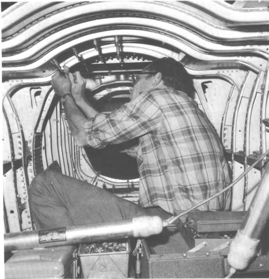
Assembler attaches cliquots, a device for pneumatic placement of screws.
