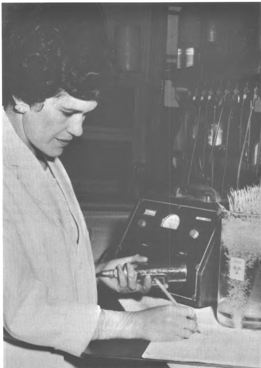
Soil scientist conducts test on barley roots with aid of ionization detector.
