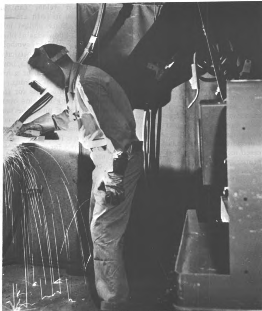
Welder operates CO 2 gas shielded welding equipment.
