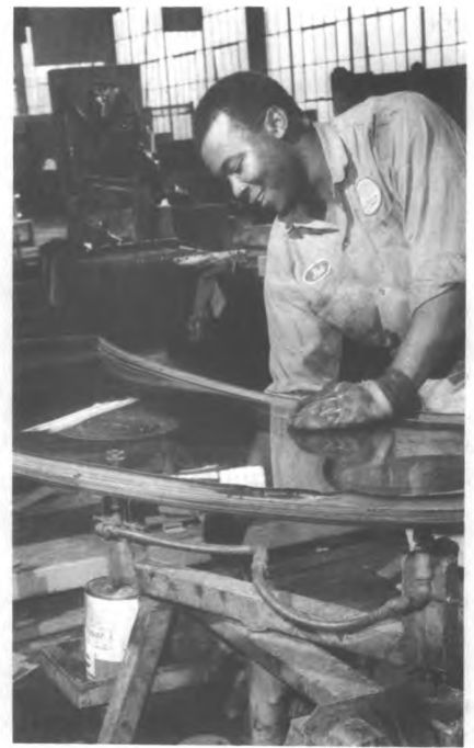
Worker places weatherstrip around windshield.
