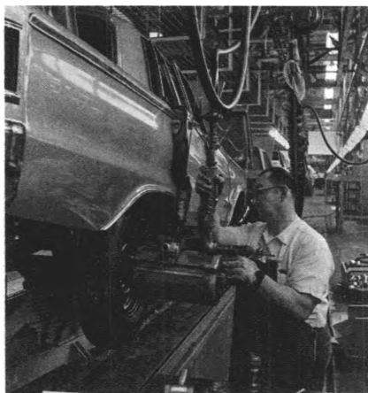
Operator tightens all wheel lugs at once with pneumatic impact wrench.
