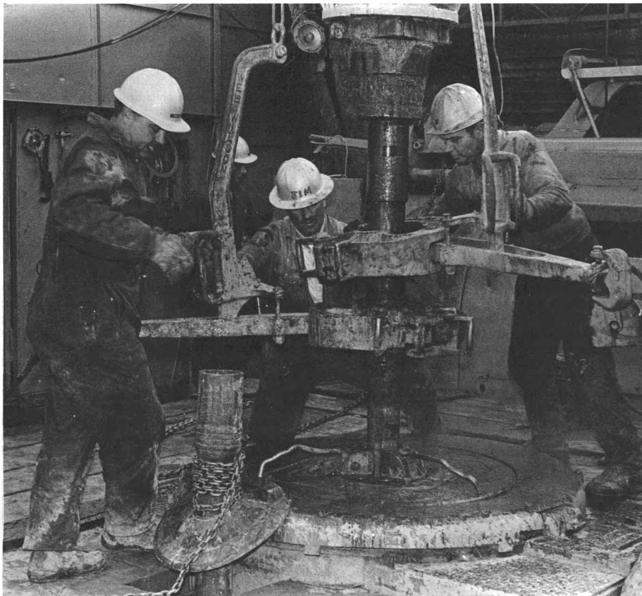
Rotary drilling crew lowers section of drill pipe.
