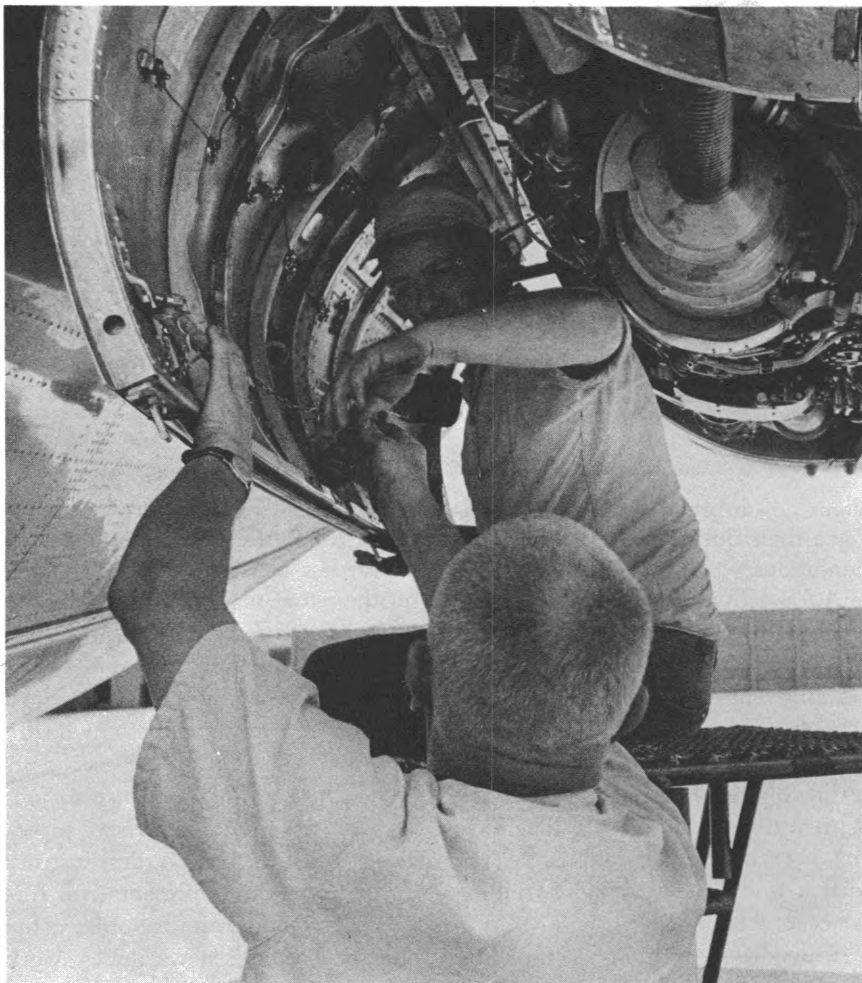
Line mechanics service engine on jet aircraft.
