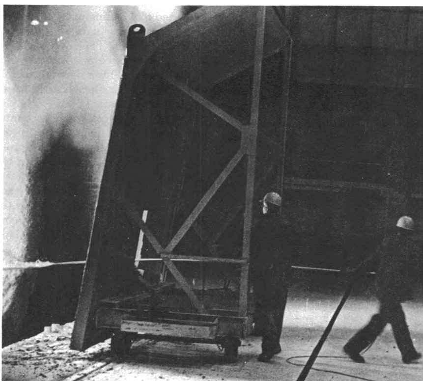
Melter helps sample steel from basic oxygen furnace.
