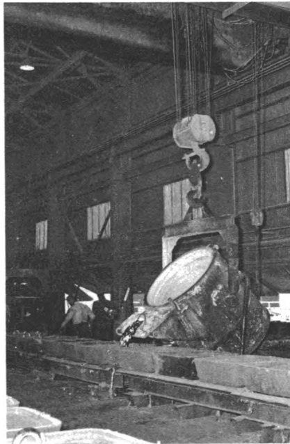
Molten aluminum is poured into 1,000-pound ingots.
