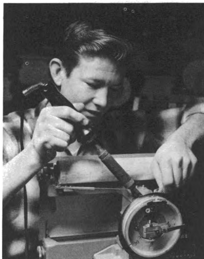
Repairman uses soldering iron to repair recording instrument.
