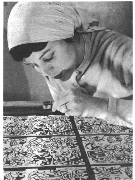
Inspector examines negative used in making circuit boards.
