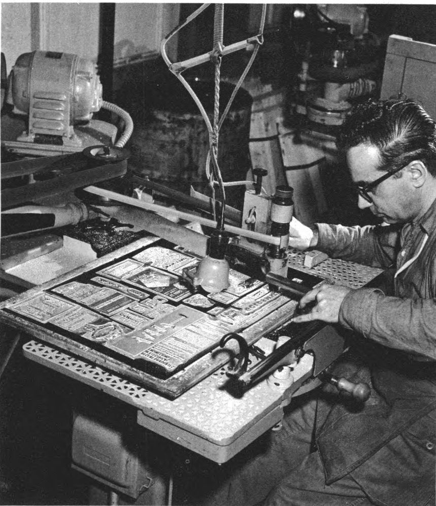
Photoengraver cuts away metal from nonprinting areas of printing plate.
