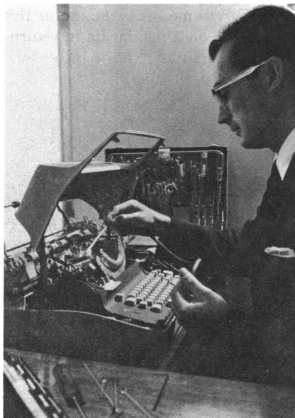
Typewriter serviceman uses air jet to remove dust and erasure particles.
