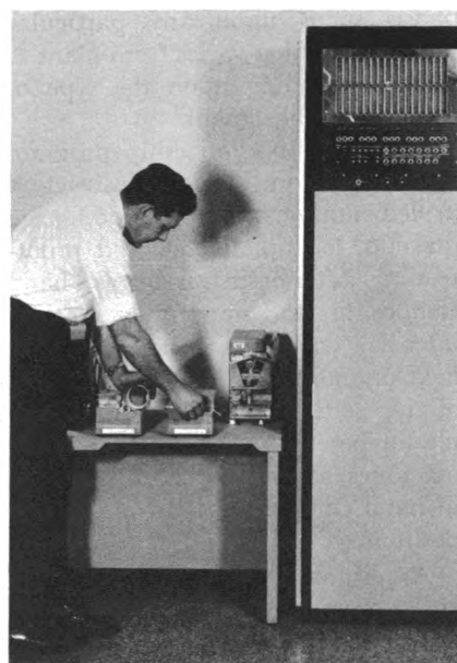
Typesetter prepares automatic linecasting machine tape for hyphenation and justification by computer.
