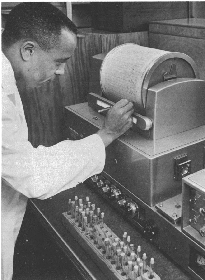
Chemist identifies absorption bands with infrared spectrometer.
