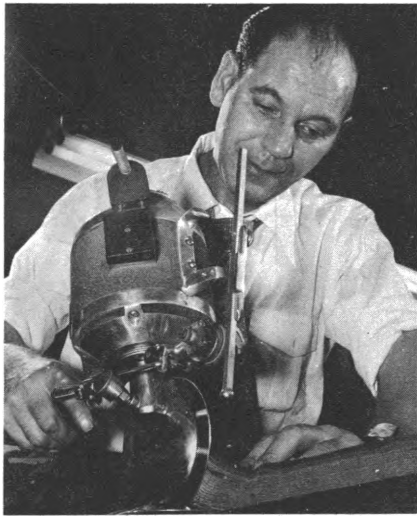
Cutter uses round knife machine to cut through many layers of cloth.
