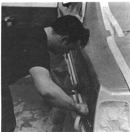
Painter covers chrome with masking tape before painting automobile.
