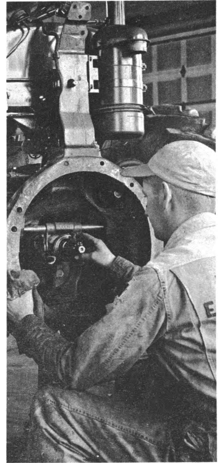
Farm equipment mechanic assembles transmission shaft of tractor.
