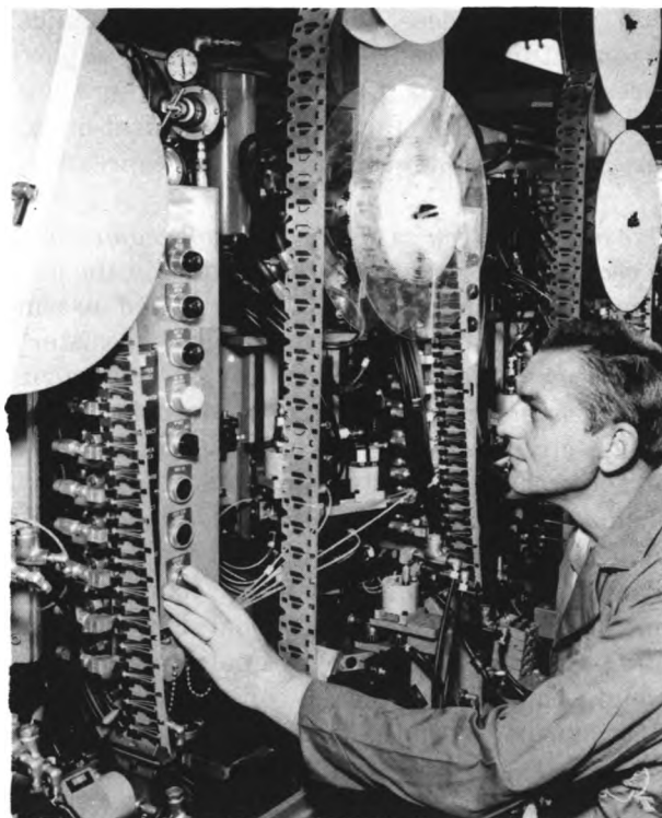
Worker monitors automatic assembly and test equipment which inserts transistors and other parts into terminal board covers.
