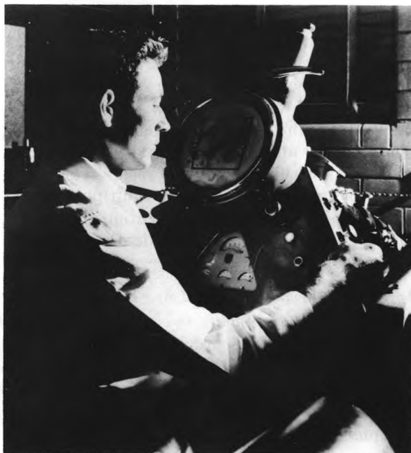
Magnifying up to 100,000 times, the electron microscope is used to aid scientific and industrial research.
