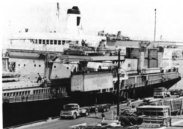
A 35-foot trailer is loaded directly from truck to deck or hold of a containership.
