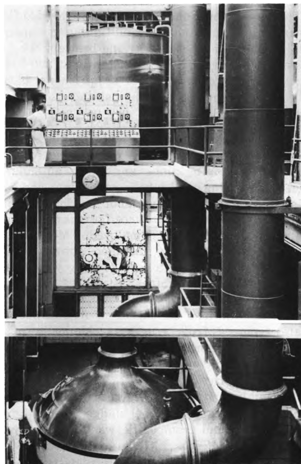
Brewery workers check cooking control board and brew kettles in an advanced brewery.
