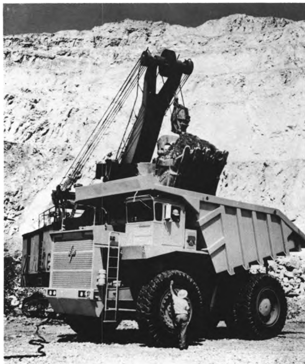
Copper ore is loaded into an 85-ton off-highway truck.
