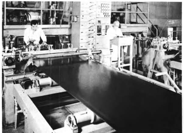
Control line worker observes processing of reconstituted tobacco sheet used as binder and wrapper in automatic cigar manufacturing.
