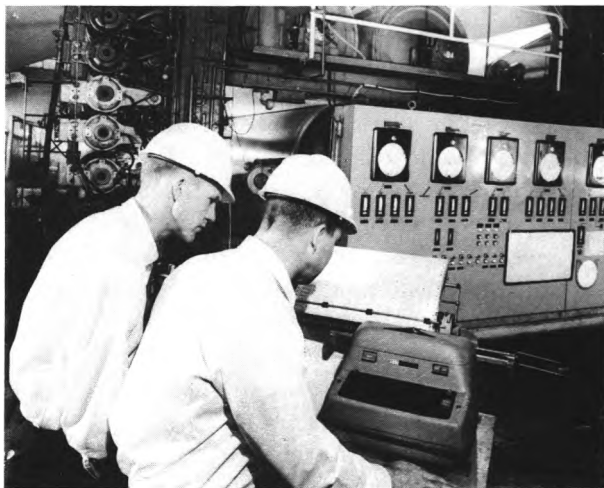
Technicians examine data provided by a computer control system installed on a paper machine.
