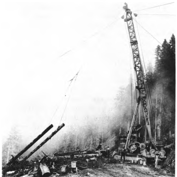
Portable tower which replaces natural spar tree is used to assemble logs for shipment to the mill.
