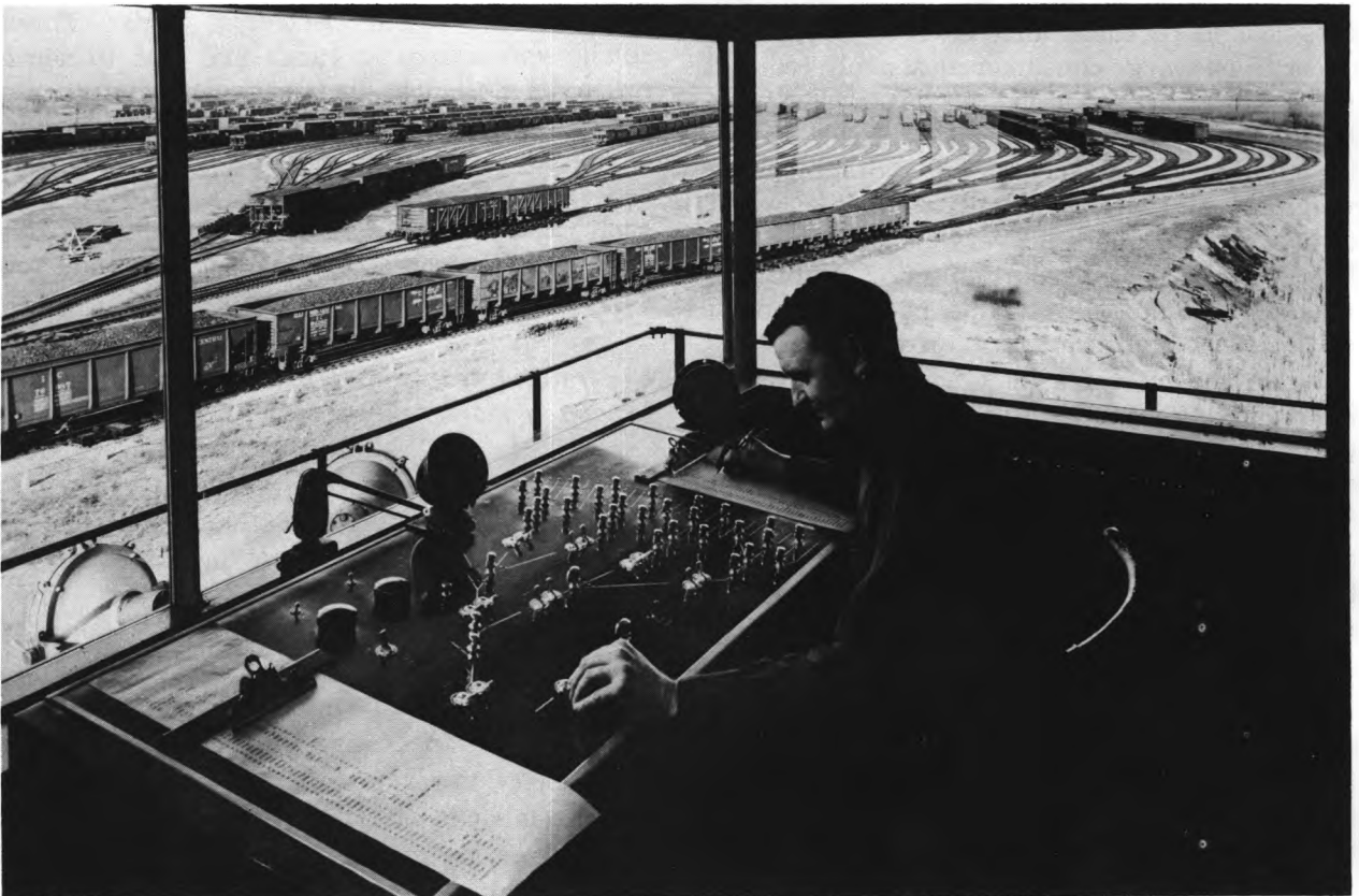
Retarder operator controls the speed of coasting freight cars in classification yard.
