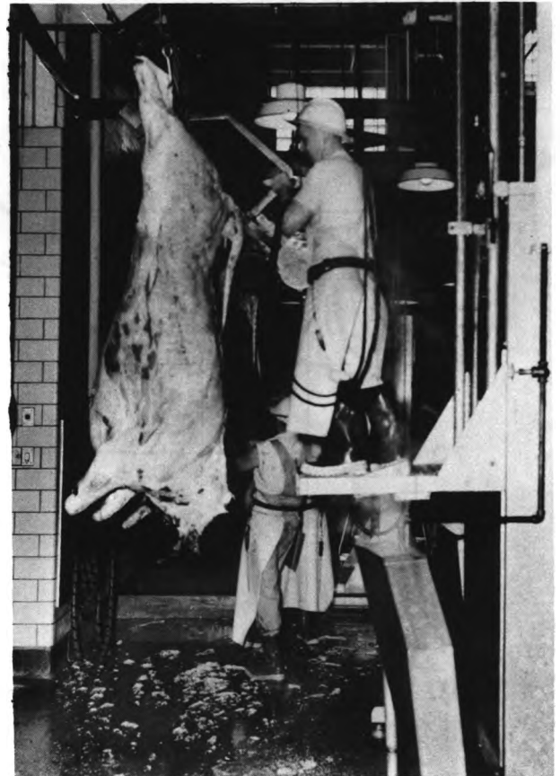
Carcass is split as it travels on rail, by worker on moving platform.
