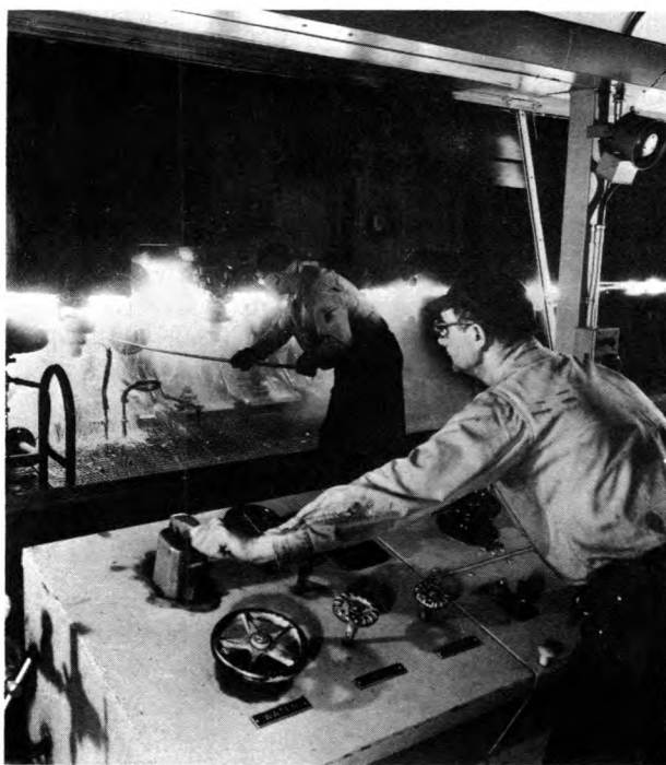
While his helper knocks off scale, speed operator (one type of roller) controls continuous butt weld pipe mill.
