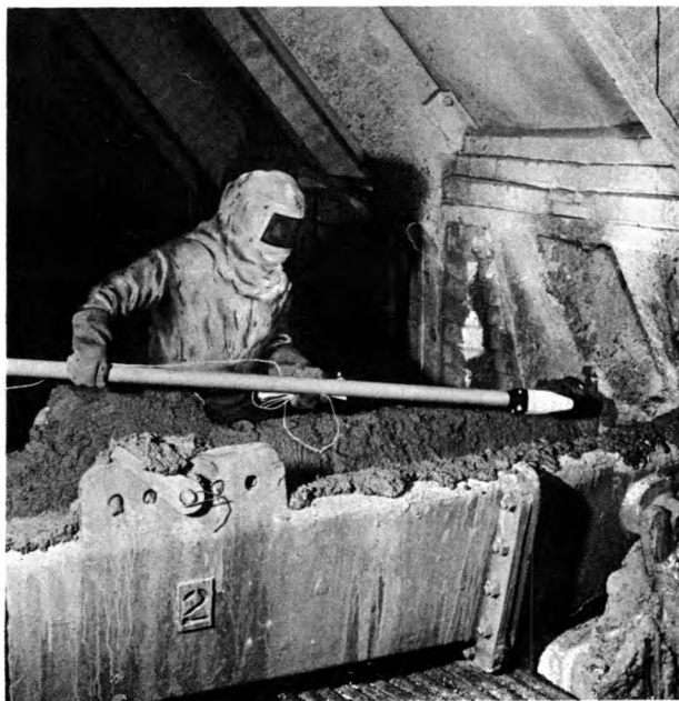
Melter's helper inserts jet tapper into open hearth furnace tap hole.
