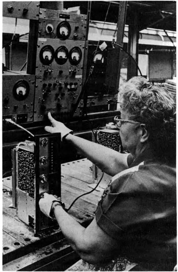
"Hot-line" tester checks solid-state circuit in high fidelity tuner.
