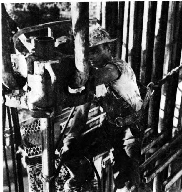
Derrickman works high above rig floor whenever pipe is hoisted from or lowered into well bore.
