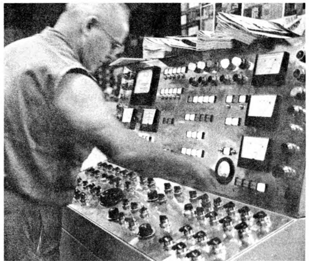
Chief pressman uses electronic console to control huge newspaper press.
