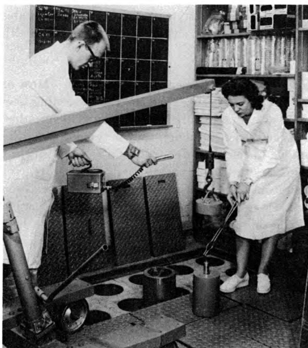
One technician monitors the radiation level while another lifts radioisotope source holder from lead "can."
