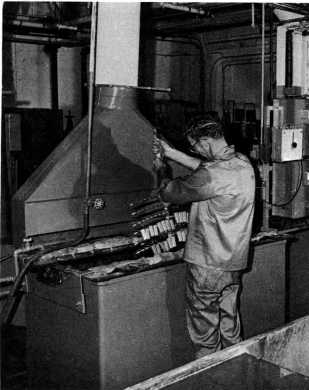
Electroplater lowers metal parts into nickel plating bath.
