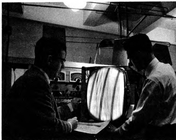
Service technicians follow schematic diagram and use modern test equipment to check television receiver.
