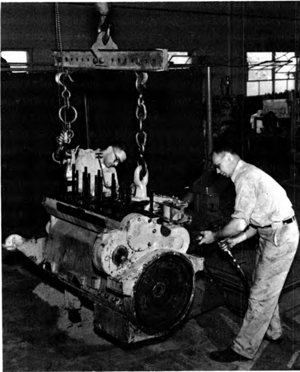
Diesel mechanics use power tools to disassemble engine.
