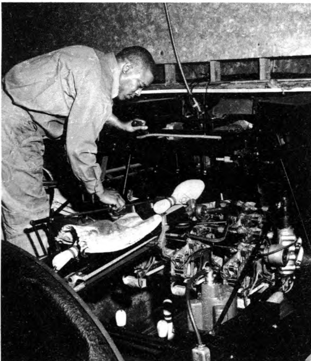
Automatic bowling machine mechanic inspects pin conveyor mechanism.
