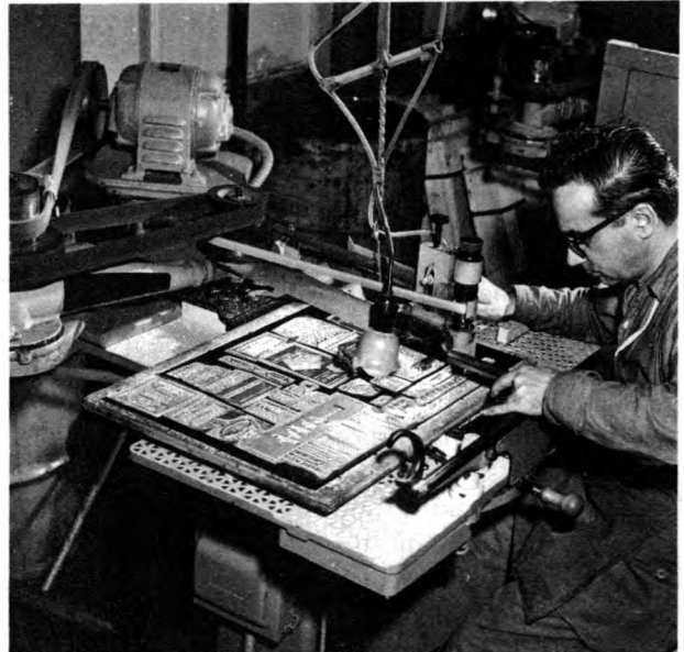
Photoengraver routs metal from nonprinting areas of printing plate.
