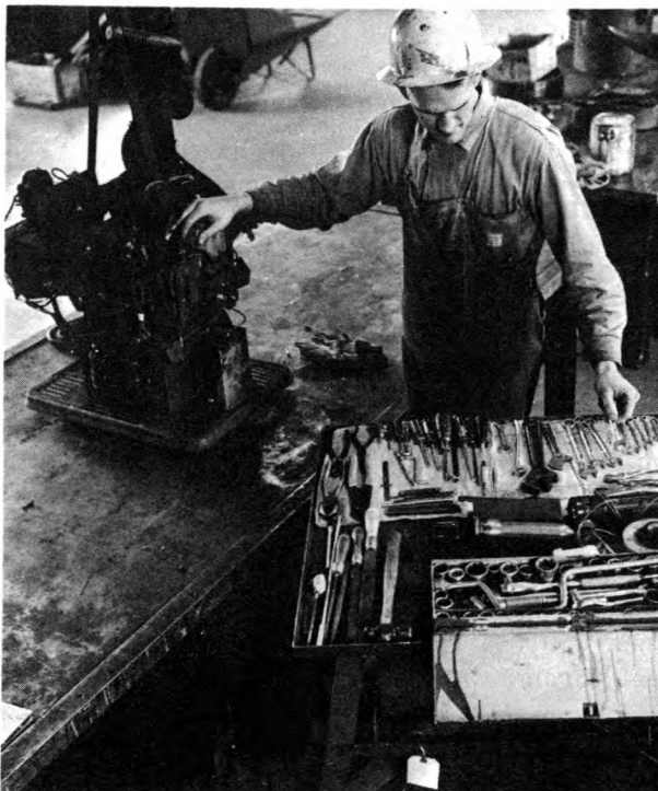
Maintenance electrician repairs welding machine.
