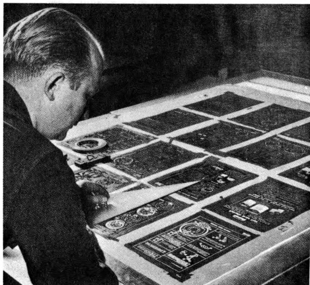
A stripper pastes type and picture negatives in a "strip-up" from which a lithographic plate will be made.
