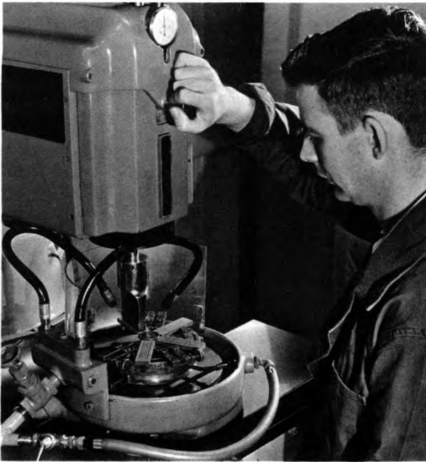
Instrument maker uses an ultrasonic machine tool.
