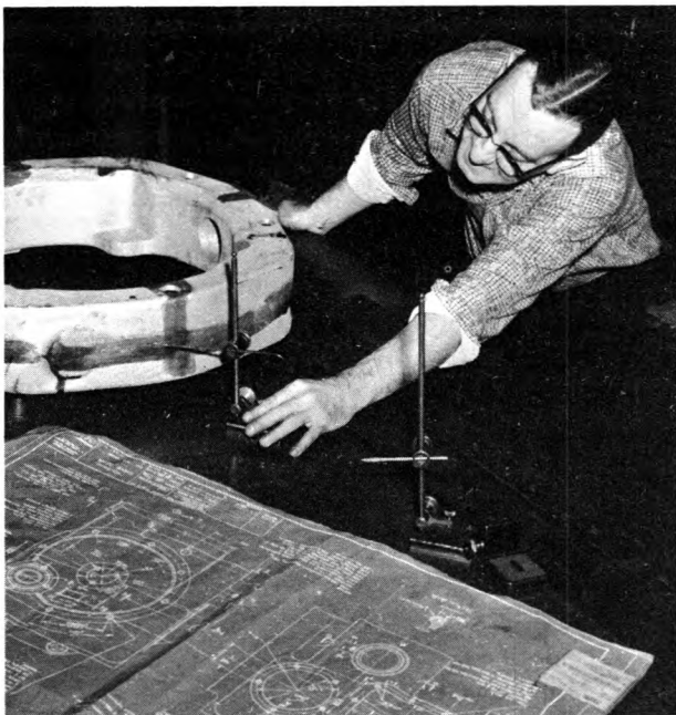
Layout man uses a surface gage to mark lines and reference points for machine tool operator.
