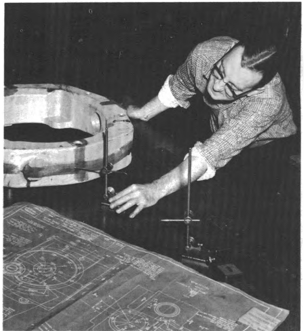
Layout man marks lines and reference points with surface gage to guide machine tool operator
