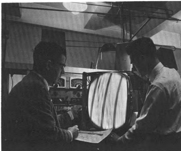
Servicemen use schematic diagram and modern test equipment to check television receiver
