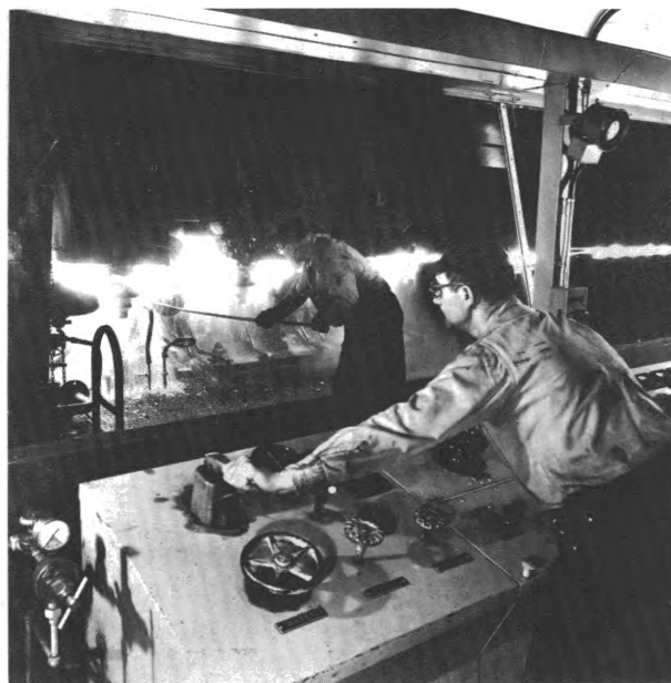
Speed operator (one type of roller) controls continuous butt weld pipe mill while helper knocks off scale
