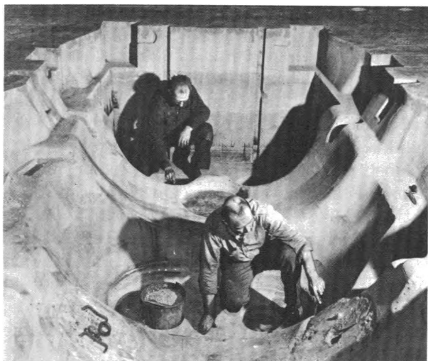
Hand molders use trowels to finish floor mold
