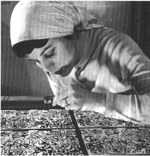
Inspector uses magnifying glass to check negative used in printing electrical circuits on circuit boards
