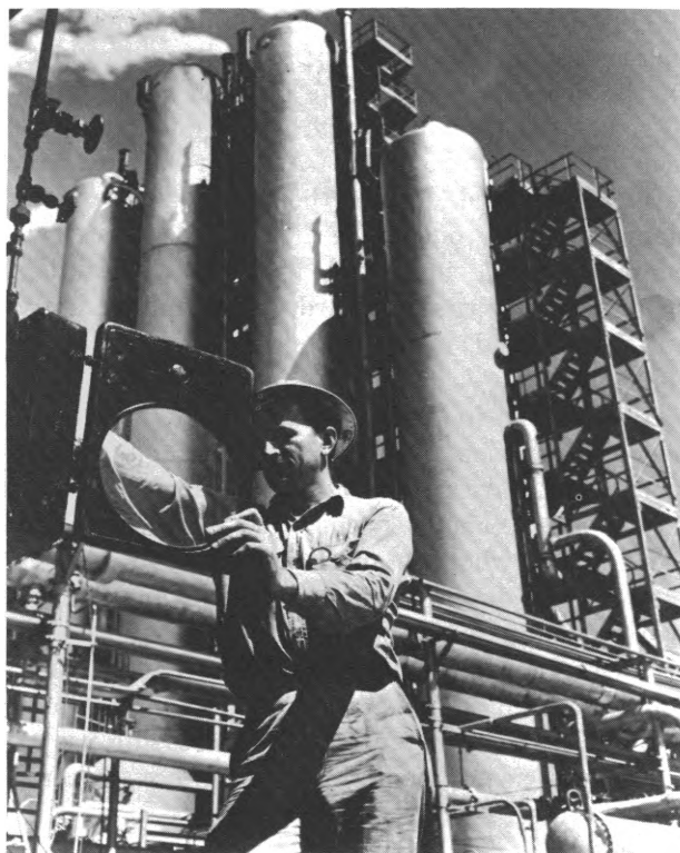
Pumpman adjusts flowmeter, one of many automatic instruments used in modern refinery
