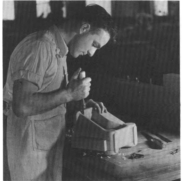
Patternmaker uses gouge to carve wood pattern
