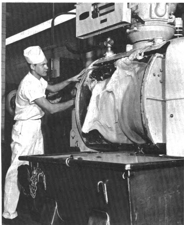
Dough mixer releases dough in trough
