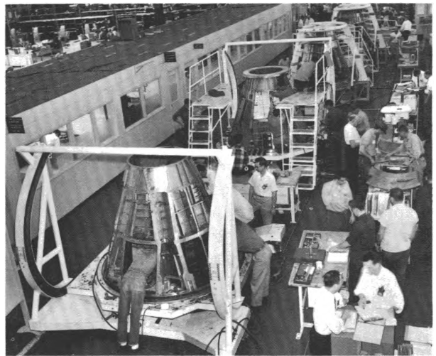
Assembly mechanics install equipment in cabin capsules for manned space exploration
