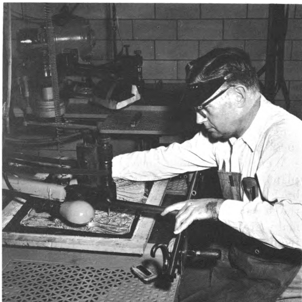
Photoengraver cuts away (routs) metal from nonprinting areas of a plate
