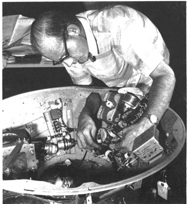
Technician wiring a rocket nose cone for a space capsule.
