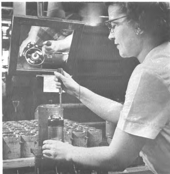
Inspector uses a mirror to help in checking brushes in a motor
