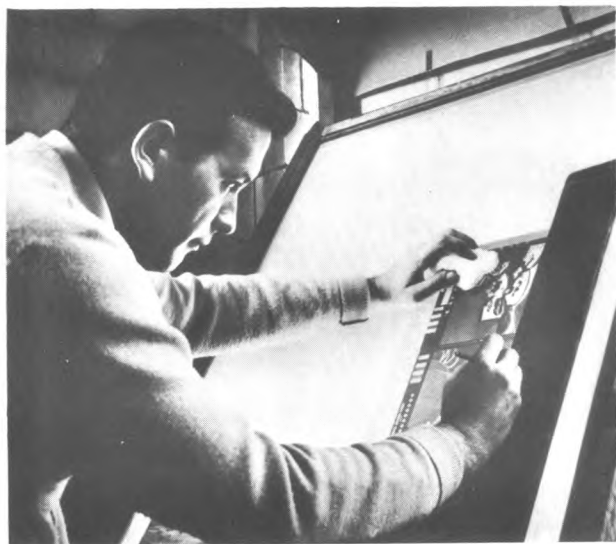
Lithographic artist sharpening image on a negative.
