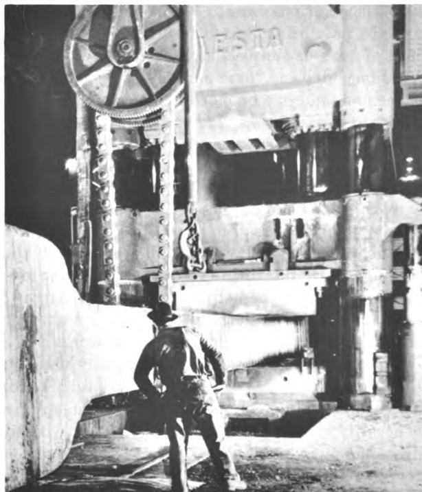
Press operator directing the forging of huge metal piece between open dies of a forging press.
