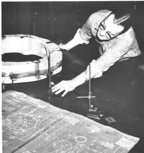
Layout man marking lines and reference points on a casting with a surface gage to guide the machine tool operator.
