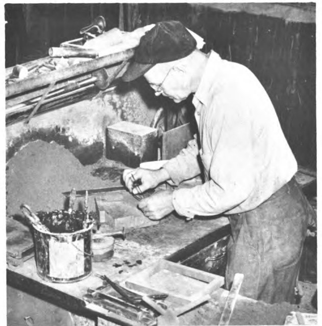
Coremaker setting reinforcing wires in sand in a core box.
