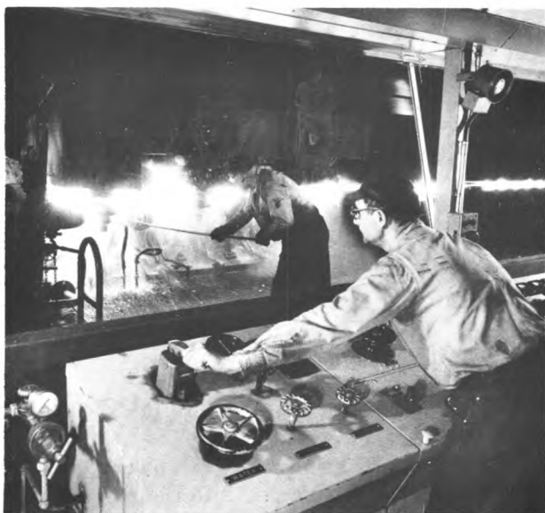
Speed operator (one type of roller) oversees the action of a butt weld pipe mill while a helper knocks off scale.
