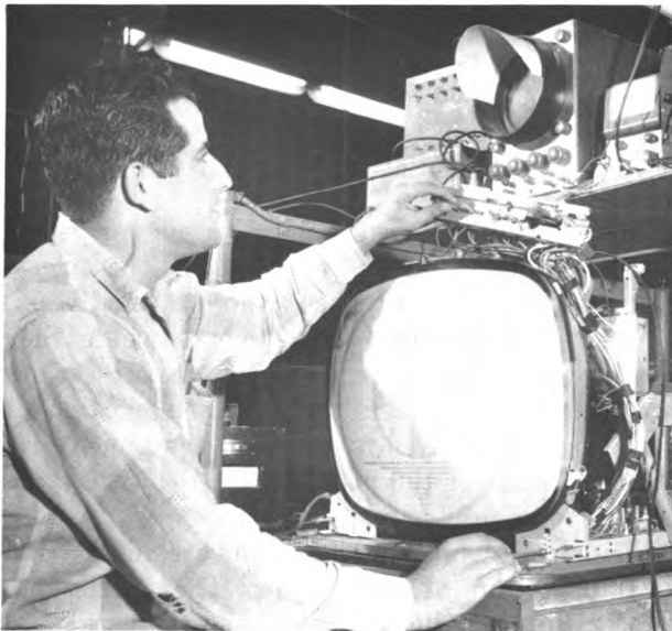
Near the end of an assembly line, a skilled electronic technician checks and adjusts the test pattern on a TV picture tube.
