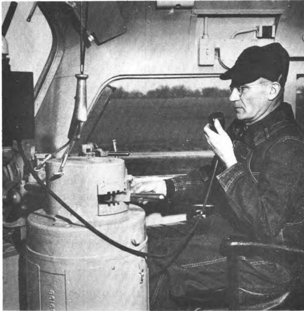
An engineer at the controls of a diesel locomotive communicates with members of the train crew by radio.
