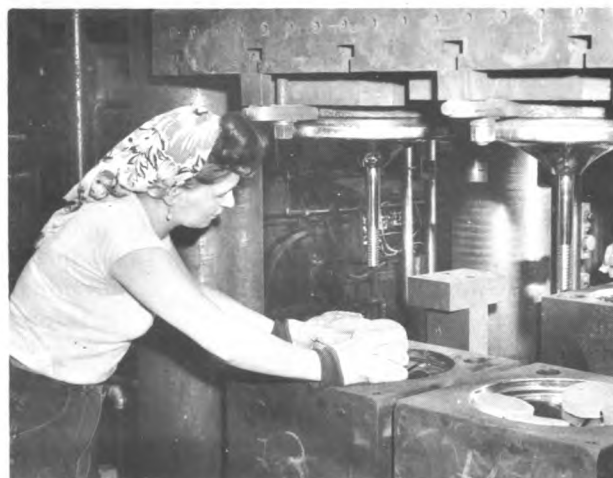
Loading preformed plastic forms into a mold to make washing machine agitators. About one-third of the employees in the plastic products industry are women.
