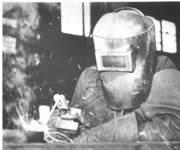
Special clothing and protective helmets guard arc welders against burns and eye injuries.
