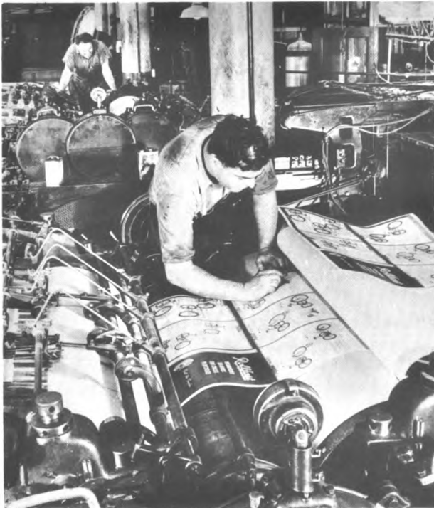
Pressman checking fidelity of press impressions—an important phase of "makeready" operations.
