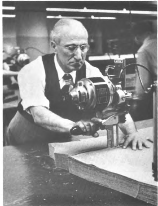
Cutter using machine to cut garment parts from marked plies of cloth.
