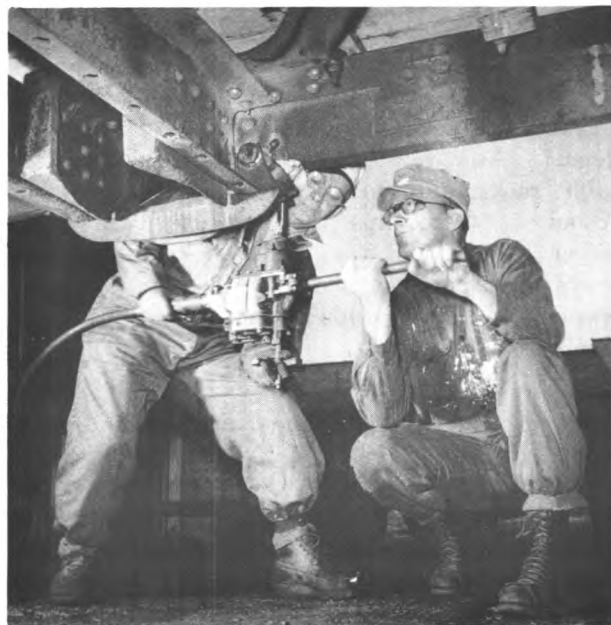
Carmen, in repairing rolling stock, use pneumatic and electrical equipment to turn bits at high speed.
