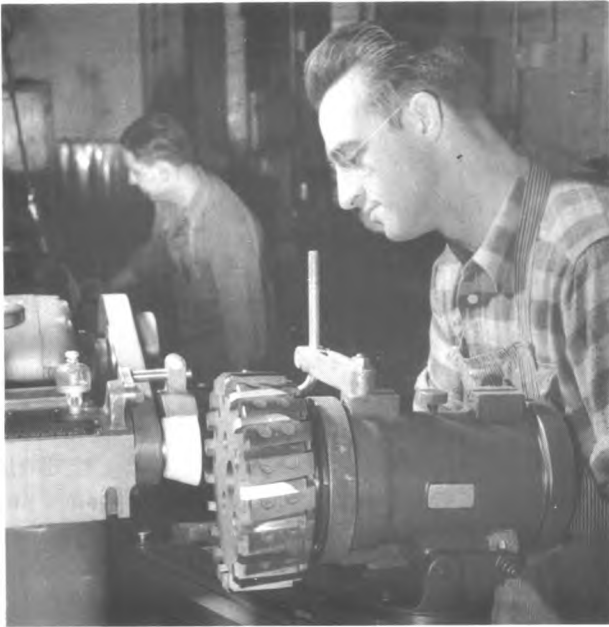
Machine tool operator grinding the surface of a metal part.
