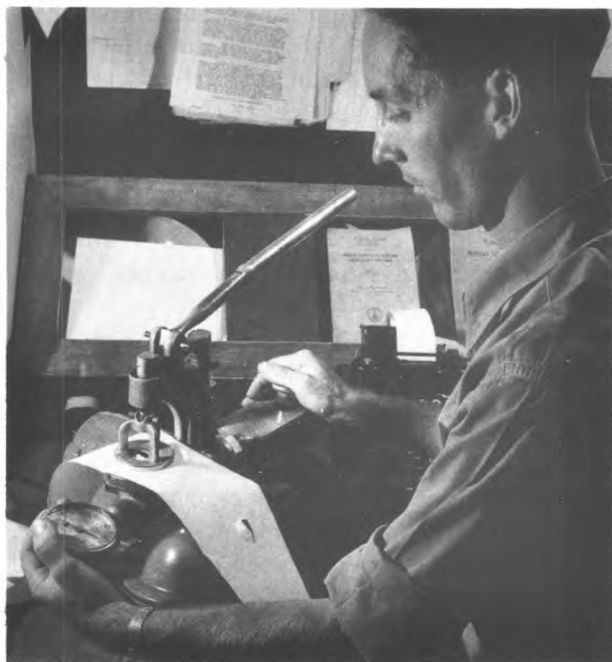
Paper inspector testing the bursting strength of a newly made sheet of paper.
