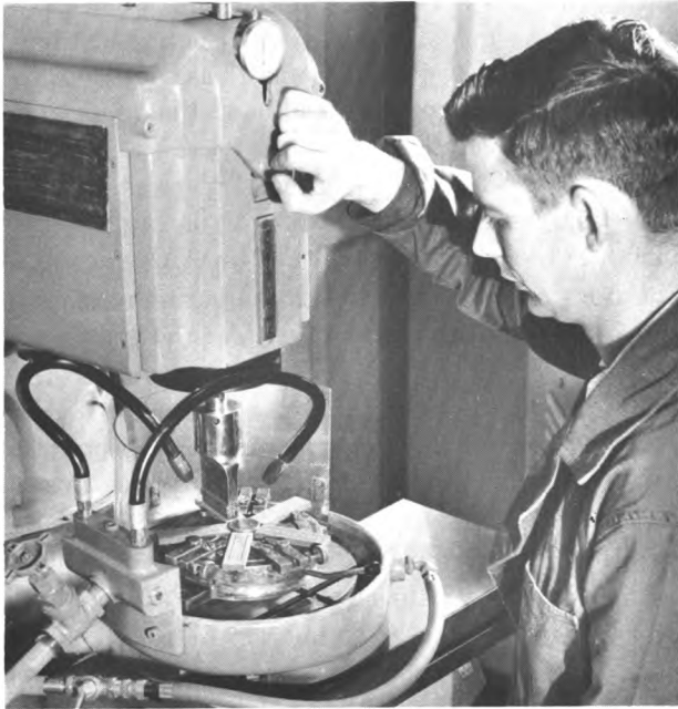
Instrument maker using ultrasonic machine tool.
