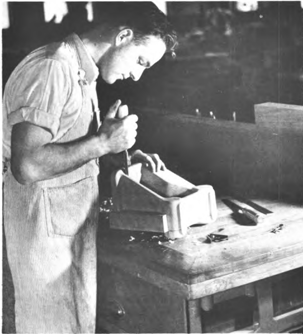
Patternmaker using a gouge to carve a round corner in a wood pattern.
