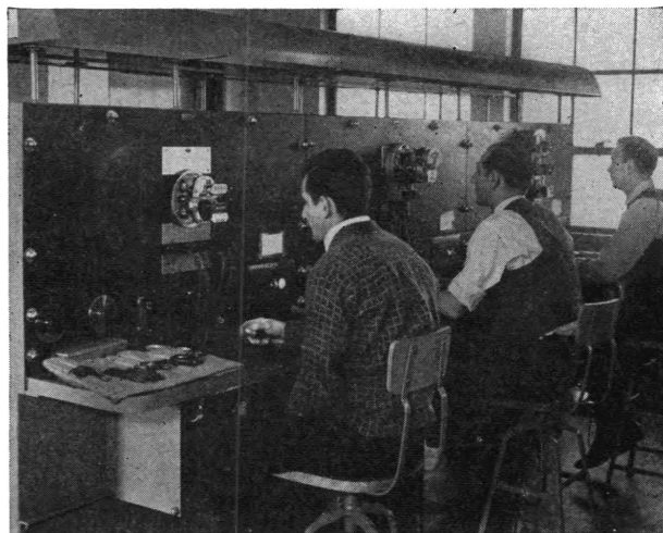
Meters are tested periodically to make sure that they are accurately measuring consumption of electricity.
