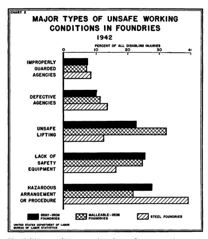
Unsafe lifting conditions constituted a much more prominent source of accidents in the malleable-iron foundries than in either the grayiron or steel foundry groups. Comparatively, these unsafe conditions were involved in 1 out of every 3 of the malleable-iron foundry injuries for which details were available, slightly less than 1 in every 4 of the gray-iron foundry injuries, and 1 in every 8 of the steel foundry injuries.
