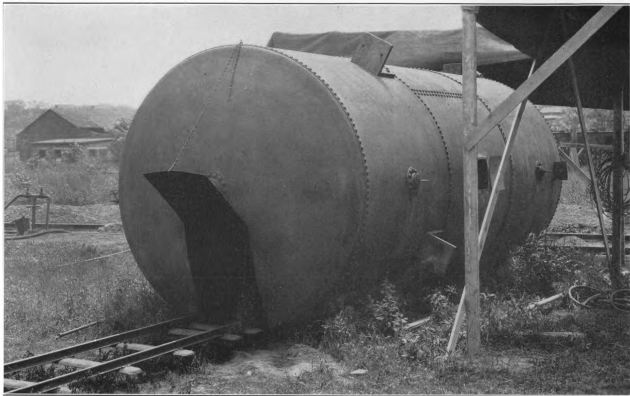
FIGURE 5.—910 cubic-foot tank used in investigating products of combustion of cellulose nitrate X-ray film negatives, showing track leading into tank for carrying into tank chemical and other testing apparatus
