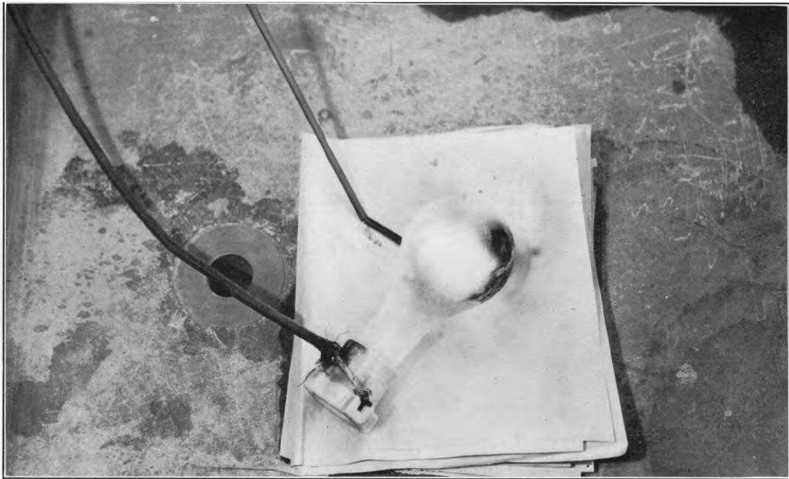
FIGURE 1.—Acetate films, eight layers inclosed in envelope, with two layers of paper between successive films. 100-watt frosted lamp was placed on negative films as shown. Temperatures were obtained by means of a thermocouple connected to a potentiometer indicator, the hot junction of the couple placed as nearly as possible at point of highest temperature of films
