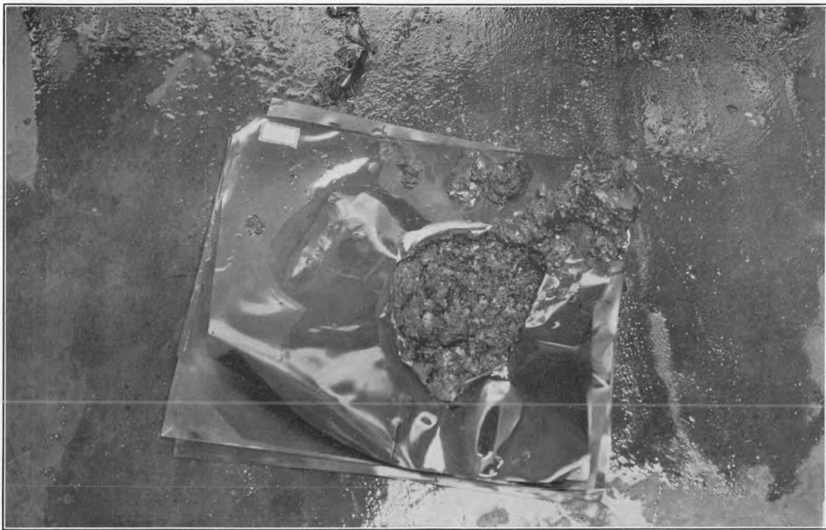
FIGURE 2.—Stack of 20 full-size cellulose nitrate film negatives in envelopes; lamp without wire guard; films ignited after exposure of 7 minutes at indicated temperature of 163° C.
