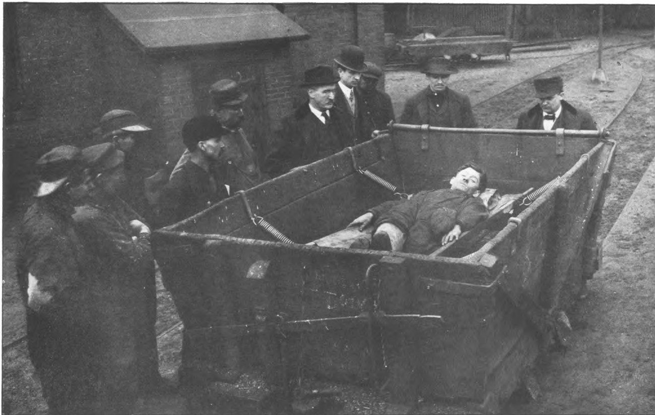
PLATE 3.—STRETCHER SUSPENDED IN MINE WAGON, WITH SPRINGS TO ABSORB ALL SHOCK AND JAR, TO TRAVEL FROM PLACE OF INJURY TO SURFACE.
