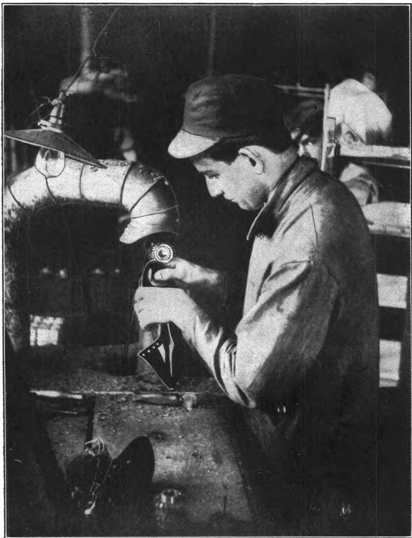
PLATE 26.—EDGE TRIMMING IN SHOE FACTORY. The dust-removal system here shown is clogged and ineffective.
