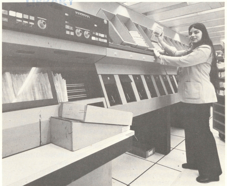
San Francisco Fed employee Christine McCoy unloads checks from one of the bank's new reader/sorters. Thanks to machines like this one, which is capable of sorting up to 110,000 items an hour, the bank processed a record 1.2 billion checks last year.
