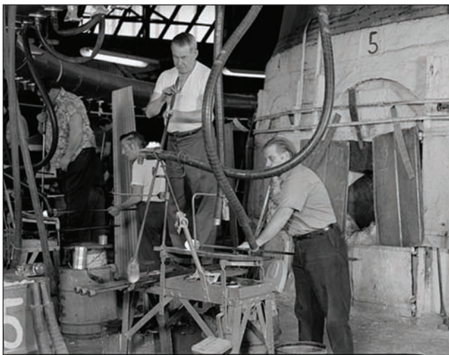
Glass blowers at Seneca Glass Co. in Morgantown, W.Va., are shown working with a bubble of hot glass in the factory's massive blowing room, with 14 clay ovens.
