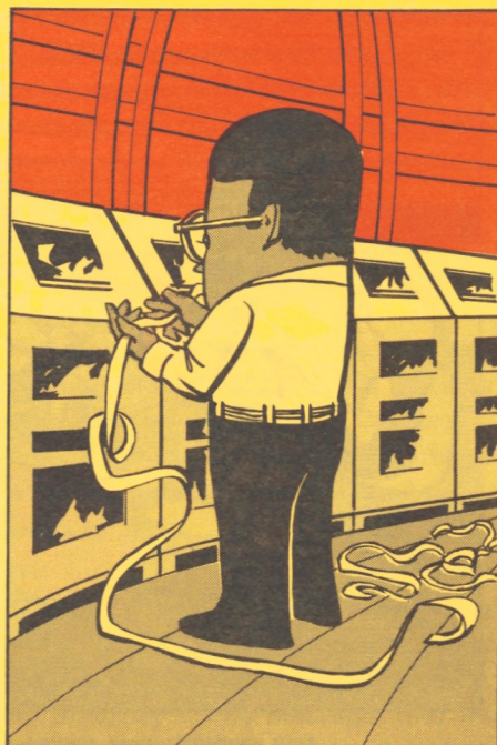
Modern teletype printers, producing 150 words a minute, supplement the monitor-console light system.
