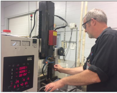
An apprentice in a HITEC apprenticeship program at Vermont Precision Tools operates an electrical discharge machining (EDM) drill to create very small precision holes on the end of a long thin part. EDM is a very precise material removal process that works on the principle of using an electric arc to quickly heat and vaporize material.
