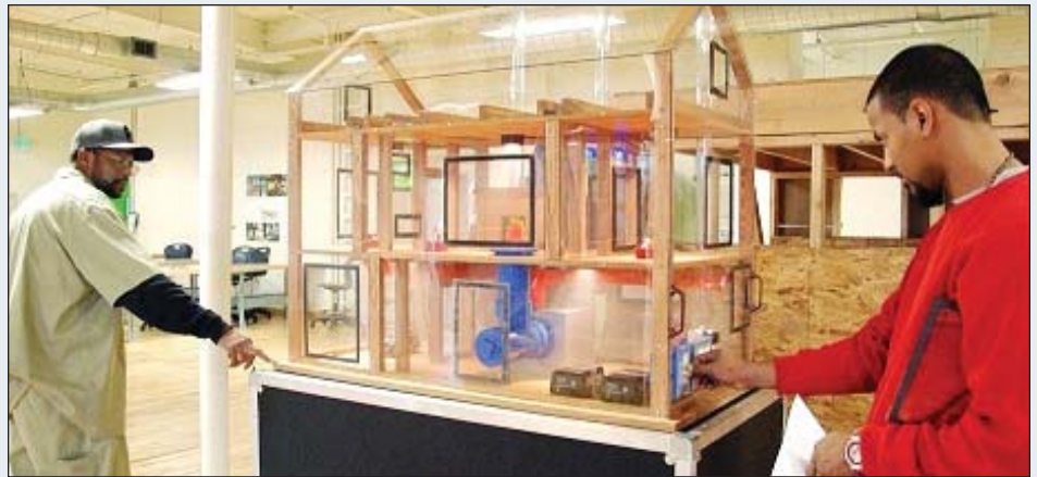
Two trainees at the Knight Green Jobs Training Center test energy efficiency in a pressurized miniature house, which has a forced-air duct system and smoke generators for the fireplace, water heater, and car exhaust.
