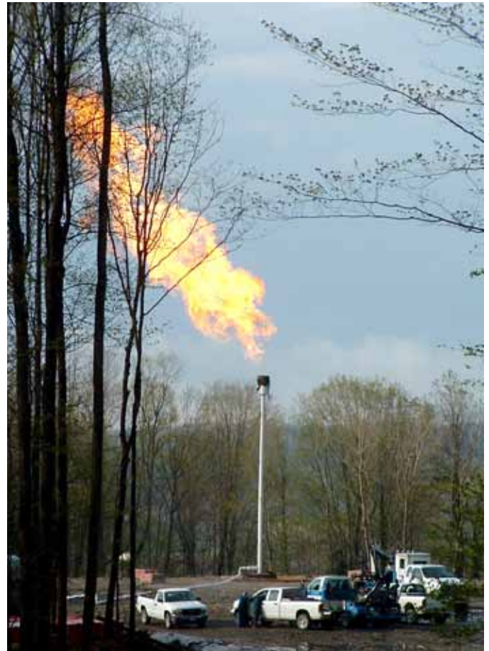
Flaring off of a well in north-central Pennsylvania after the completion of the hydraulic fracturing process.
