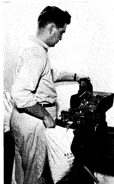
STEEL PENNIES are here being removed with an electro-magnet as their copper counterparts continue on through the counting machine into the sack. At top speed, 3,000 coins per minute, the counting machines operate with machine gun rapidity.
