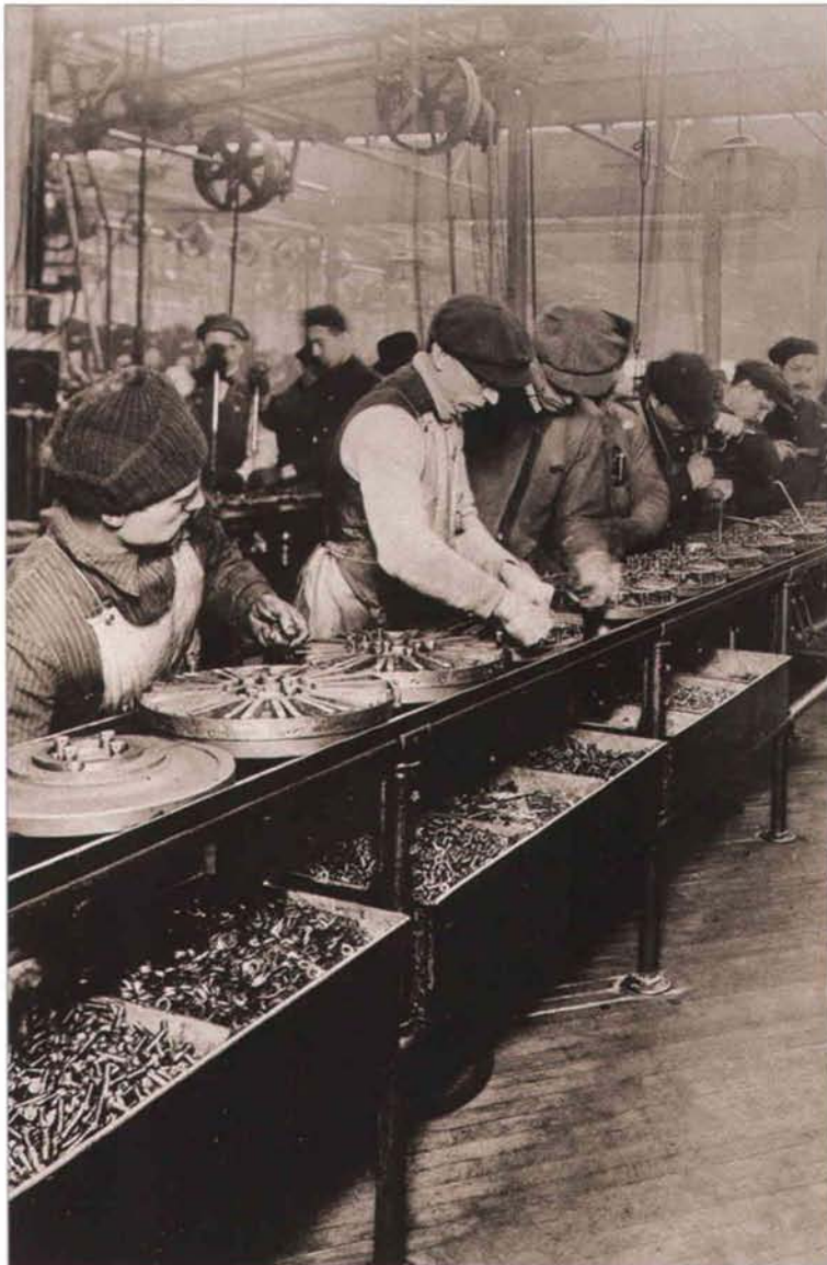
This flywheel assembly process at a Ford plant, circa 1913, was typical of the kind of repetitive task that defined the early Industrial Age.
