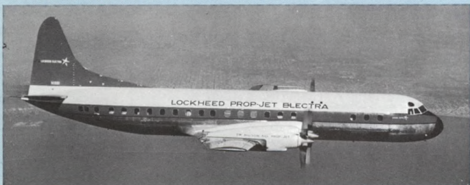
Lockheed Electra L-188 (turboprop): 1959, '61; 66-91 pass.; 400 mph; 57 tons; medium range
