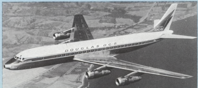
DC-8 series: 1959 to date; 112-250 pass.; 600 mph; 137-169 tons; long range
