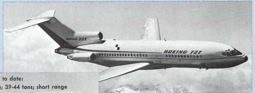
Boeing 727 series (three jets): 1964 to date: 91-170 pass.; 600 mph; 81-85 tons; medium range
