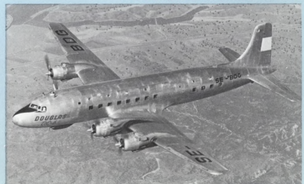
DC-6 series: 1947, '51; 52-74 pass.; 300-315 mph; 50 tons; medium/long range
