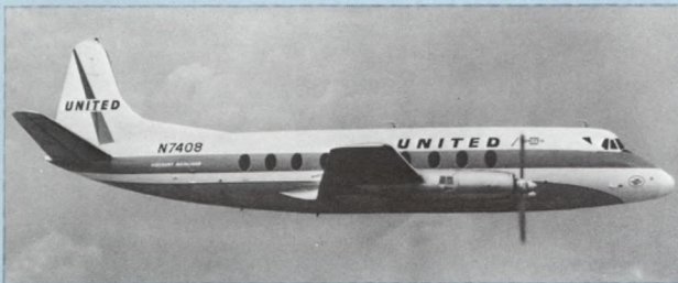
Vickers Viscount 700, 800: (British turboprop): 1955; 44-70 pass.; 320-350 mph; 32 tons; medium range
