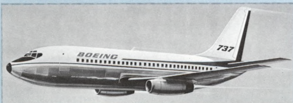
Boeing 737 series (under development): 1967; 99-113 pass.; 550 mph; 43-49 tons; short range
