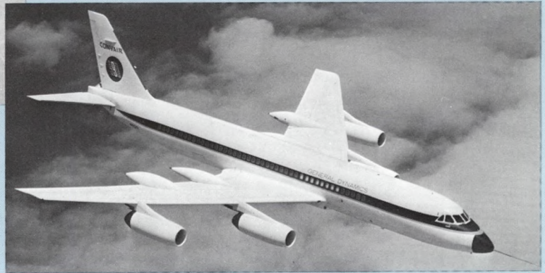
Convair 900: 1960, '62; 84-121 pass.; 600 mph; 97-120 tons; medium/long range Convair 880 (without wing pods)
