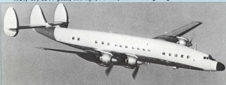
Lockheed Constellation: 1946; 44-64 pass.; 300 mph; 53 tons; medium/long range Super Constellation (similar, but larger): 1951, '57; 63-99 pass.; 350 mph; 78 tons; medium/long range
