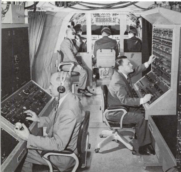
Elaborate electronic flight simulators help to train pilots and engineers in procedures
