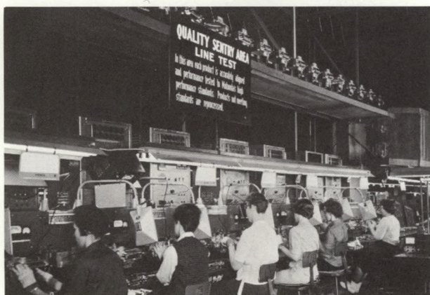
Car radios made in Quincy, Illinois, are given quality test checkout
