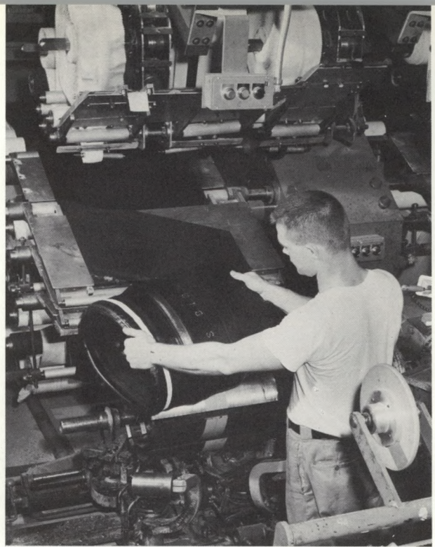
"Green" tire is removed from tire-building machine in new factory near Fort Wayne
