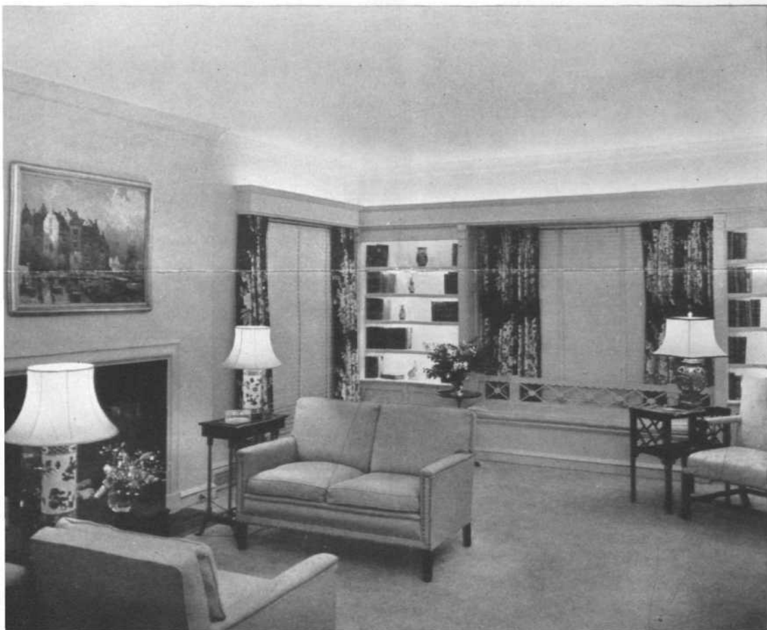
Concealed fluorescent lighting, like that in the cove and bookshelves of this living room, is one of the improved lighting arrangements for tomorrow's home. General Electric provided the fluorescent and other lights for the fixtures in this interior.
