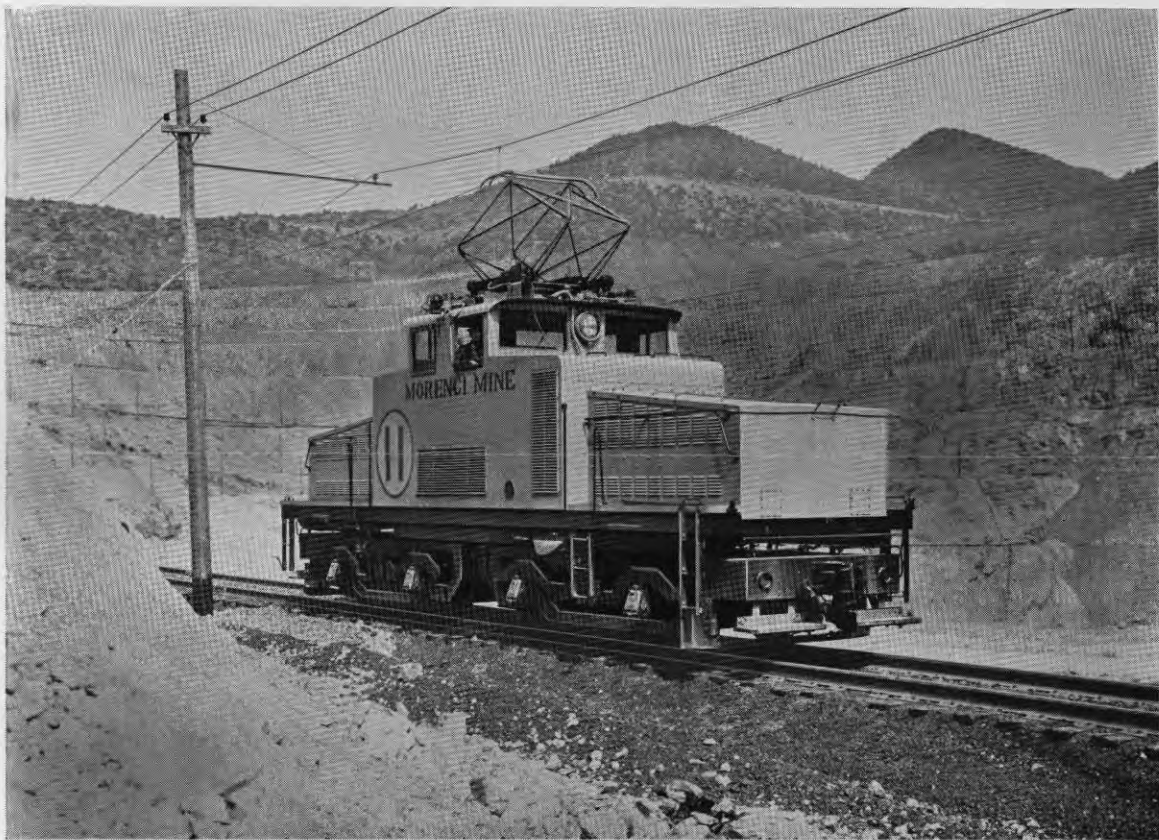
One of the electric locomotives to be used for haulage between the Open Pit Mine and the Reduction Works.
