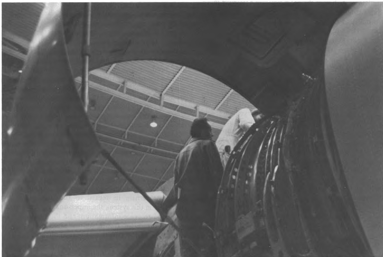
Mechanics doing maintenance on engine of wide-body jet. These engines produce more thrust with lower fuel consumption per pound of thrust by using new powerplant technology.
